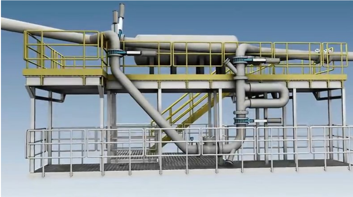
Figure 3: Installation of a Coriolis flowmeter on a conventional drilling rig using the Schlumberger flag kick detection system. It can be seen that the pipe coming out of the bell nipple splits into the measuring line and the bypass line used if the flowmeter is clogged or under maintenance. The switching between the lines can be controlled by the driller via the electric valves. The flowmeter is installed in a flag orientation to not allow accumulation of gas bubbles and solids in the measuring tube (Schlumberger FLAG Product Video 2015).
