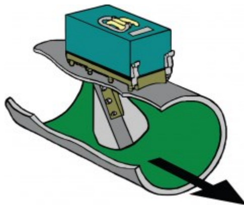
Figure 15: Typical paddle flowmeter in a partially filled pipe flow channel (Mitchell 2006).
