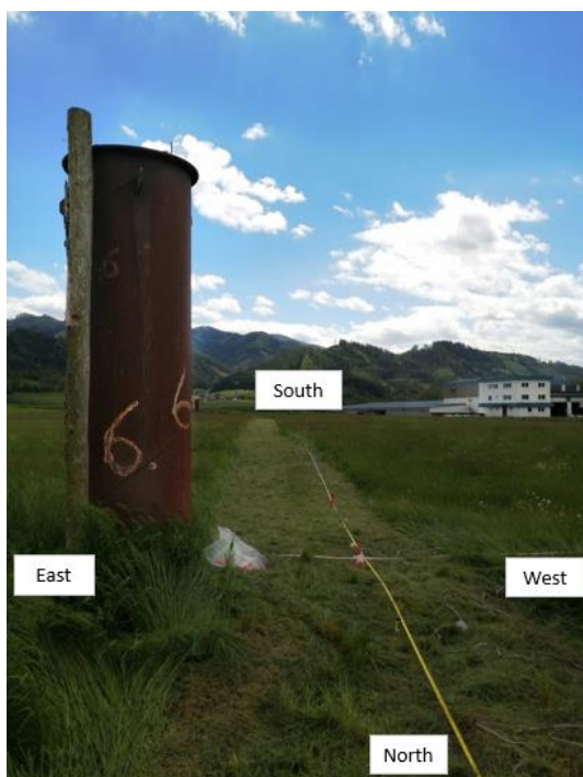
Figure 15: Showing the crossing of the profile lines directly next to the gas dome which was the metal target for detecting IP responses.
