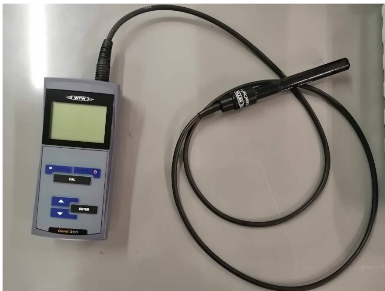
Figure 26: The WTW TetraCond 3110 SET1 meter used for the temperature and conductivity measurements of the water in the tank is shown.
