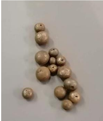
Figure 23: Example photo of the iron granule installed in the tank, which serves as a metallic detection target.
