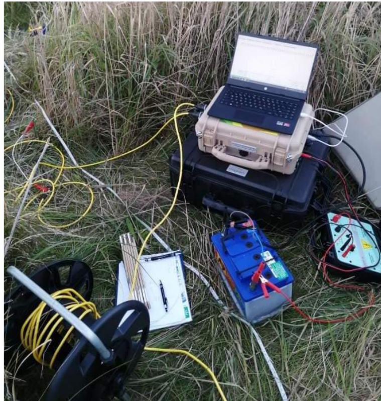
Figure 21: Showing a typical measurement setup with the Mangusta System MC 24/144E, associated current control unit as well as the measurement computer and external current supply.
