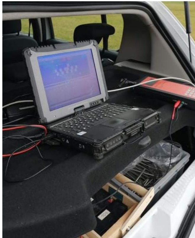
Figure 20: Representation of the measurement setup for a geoelectric measurement with the 4 point light 10W from Lippmann.
