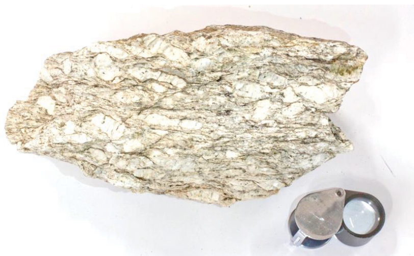
Figure 25: Sample (04-18) of leucocratic Granatspitz gneiss and the orthogneiss occurring at Messelingkogel characterized by cm-sized feldspar. The magnifier has a diameter of 2.5 cm.
