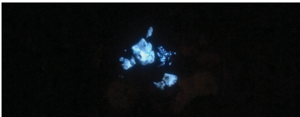
Figure 23: Blue luminescent scheelite crystal with a size of 8 mm for the large crystal. The very bright centre of the large grain is the yellow luminescing core. The quartz vein trends from left to right in the picture.
