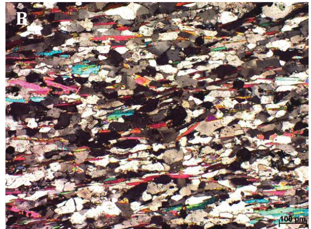
Figure 36: Photomicrographs of thin section of sample 04-09. The rock contains a significant amount of garnet. A Garnet, biotite and a roundish apatite grain in quartz-feldspar matrix; IIN. B Typical fabric of this rock under crossed nicols. Biotite is perfectly aligned in the foliation. Most black grains are isotropic garnet.
