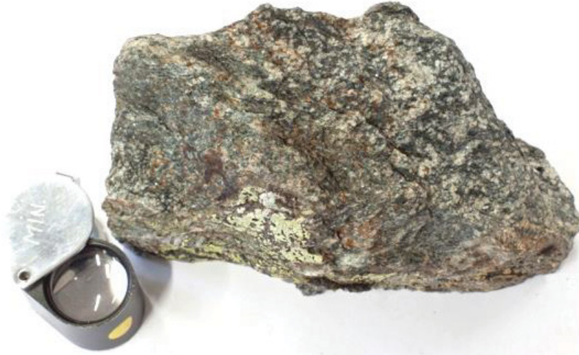
Figure 48: Hand specimen of Weinbühl amphibolite from mountain Weinbichl. The diameter of the magnifier is 2.5 cm.
