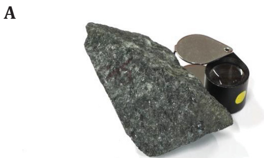
Figure 37: Photographs of green hornblende fels hand specimen. A Sample 04-04. B Sample 06-09. The magnifier has a diameter of 2.5 cm.
