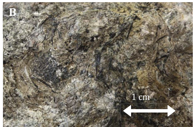
Figure 42: Hand specimen of actinolite-rich schist from west-flank of Hochgasser (sample 04-04). A Dark green actinolite schist with mm-size irregular quartz masses. B Stalky actinolite crystals with length of more than 1 cm.
