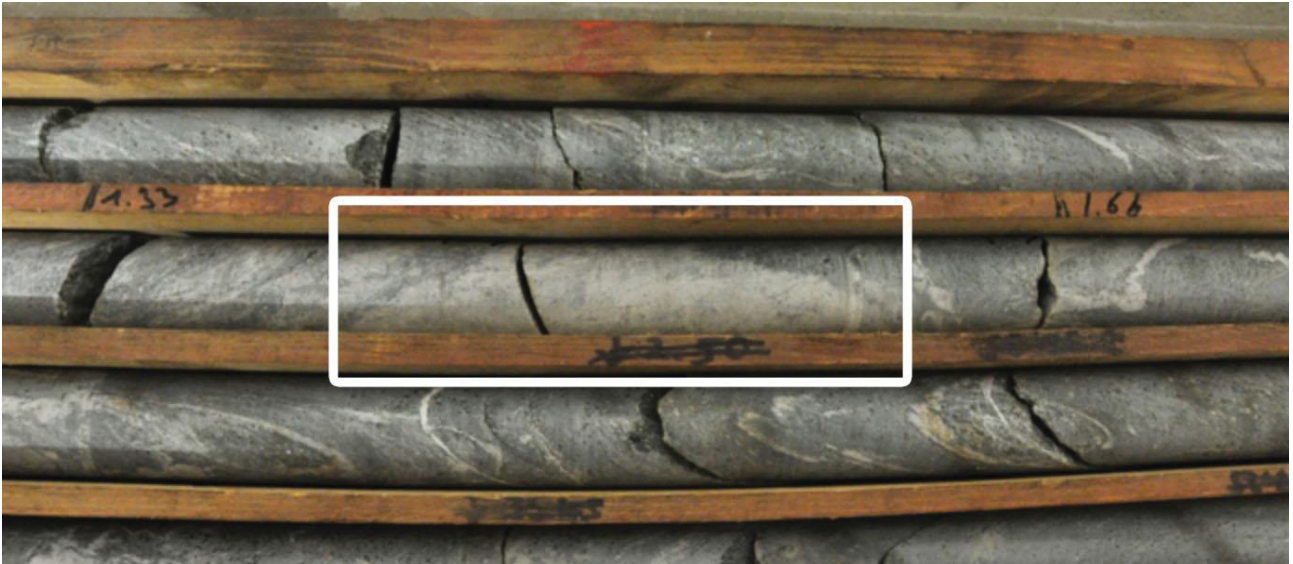
Figure 4: Drill core with calc-silicate rocks within amphibolite, Felbertal WOZ. Sample 08-01 is from drill hole UB437, 1.33-1.66m.
