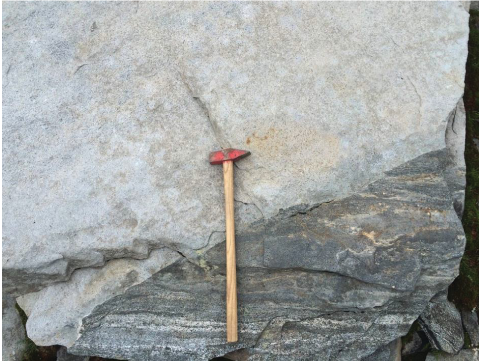
Figure 38: Intrusive contact between light hornblende-biotite gneiss and banded amphibolite. Location of the block is N47.143012, E012.506974 (around 350 m W of Messelingscharte).
