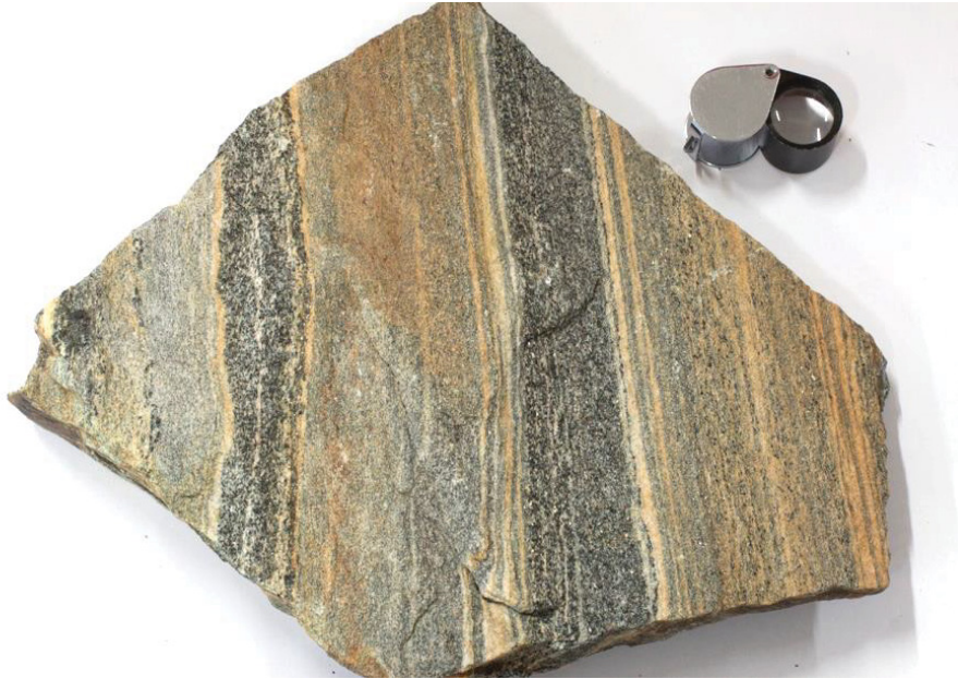
Figure 33: Hand specimen (sample 04-01) of banded amphibolite. The grain size of hornblende varies strongly between different bands. The thick hornblende-rich layer display a coarser grain size of hornblende compared to thin plagioclase-rich layers. The sample was taken closely to the northern end of Grauer See. The magnifier has a diameter of 2.5 cm.
