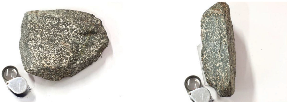
Figure 31: Hand specimen (sample 02-10) of a typical slightly foliated, coarse-grained amphibolite. The rock shows a weak foliation in cross-section. The hand lens has a diameter of 2.5 cm.
