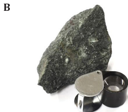
Figure 37: Photographs of green hornblende fels hand specimen. A Sample 04-04. B Sample 06-09. The magnifier has a diameter of 2.5 cm.
