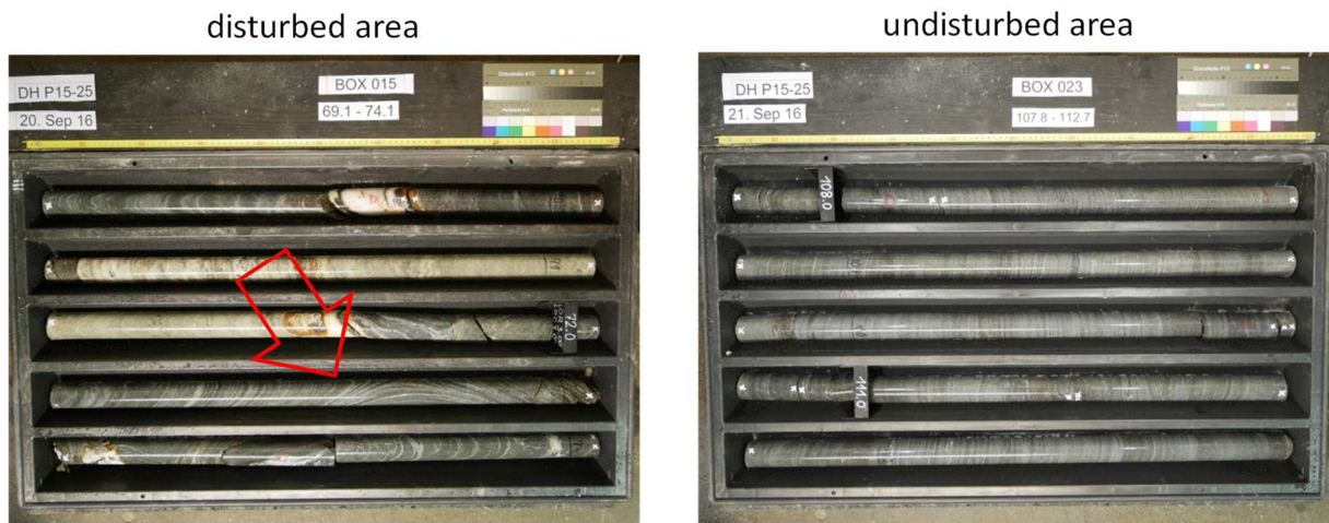
Figure 58: Examples of drill log images illustrating irregularity zone of P15-25.
