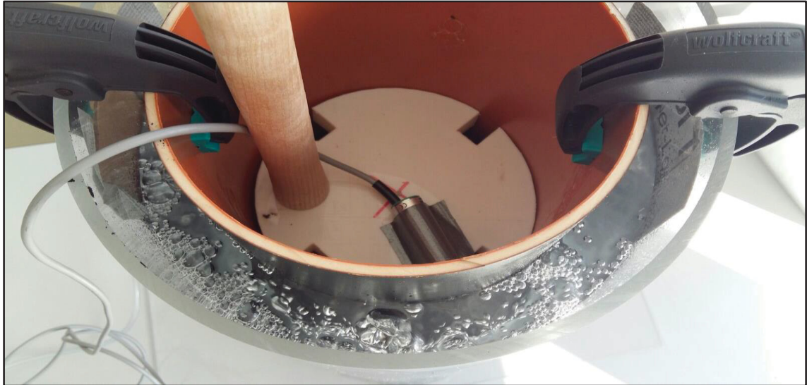
Figure 62: CJ8 – 18GM – E2 capacitive sensor during gas influx experiment
