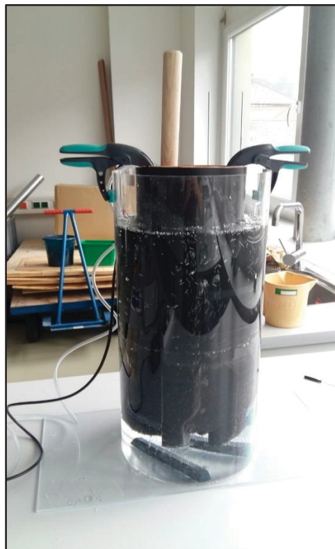
Figure 59: Conditions of artificial testing facility during gas influx entering the wellbore
