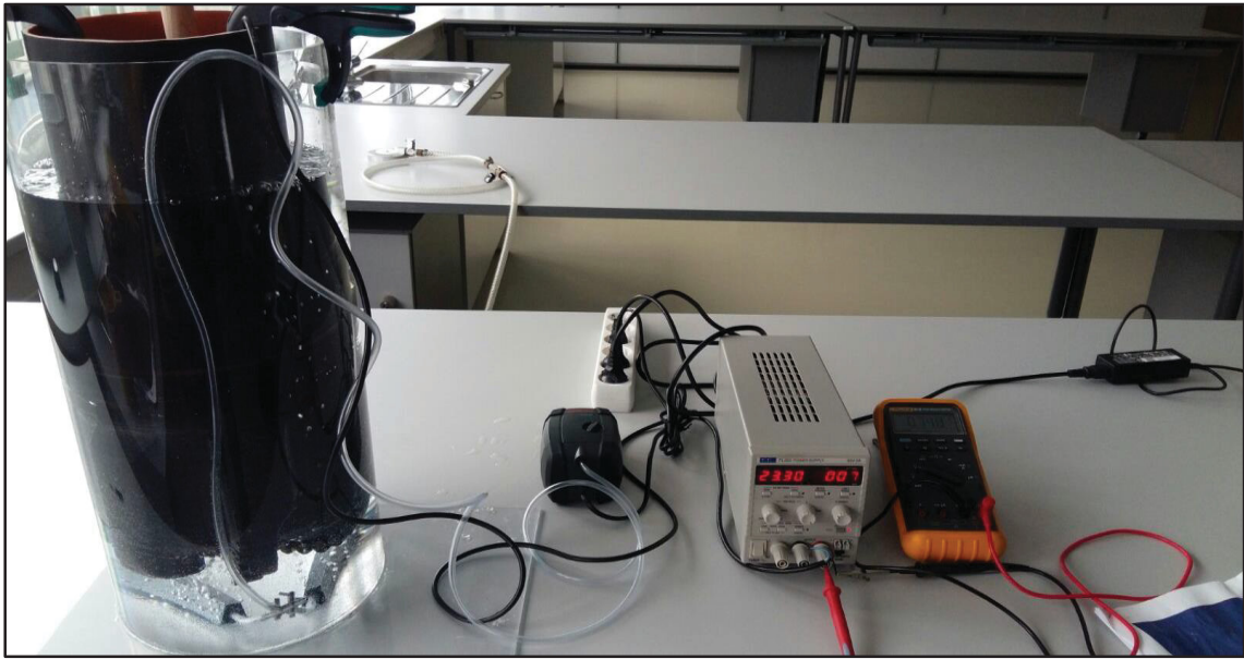
Figure 56: Workplace that experiments were conducted and the initial artificial wellbore facility connect with power supply and multimeter
