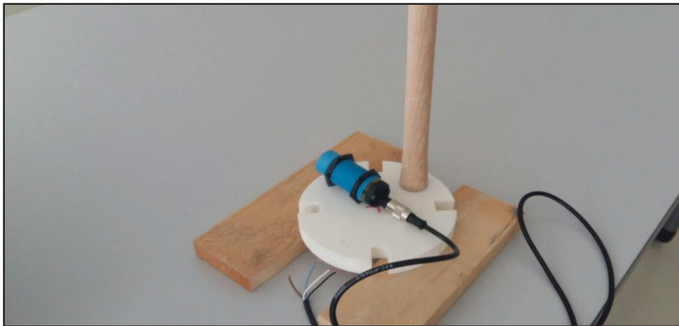
Figure 53: Sensor installation in the special base
