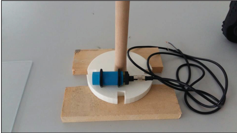
Figure 45: Special inside base for sensor installation
