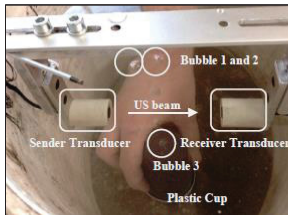
Figure 32: Placement of sender and receiver during the experiments (Kutas 2016)
