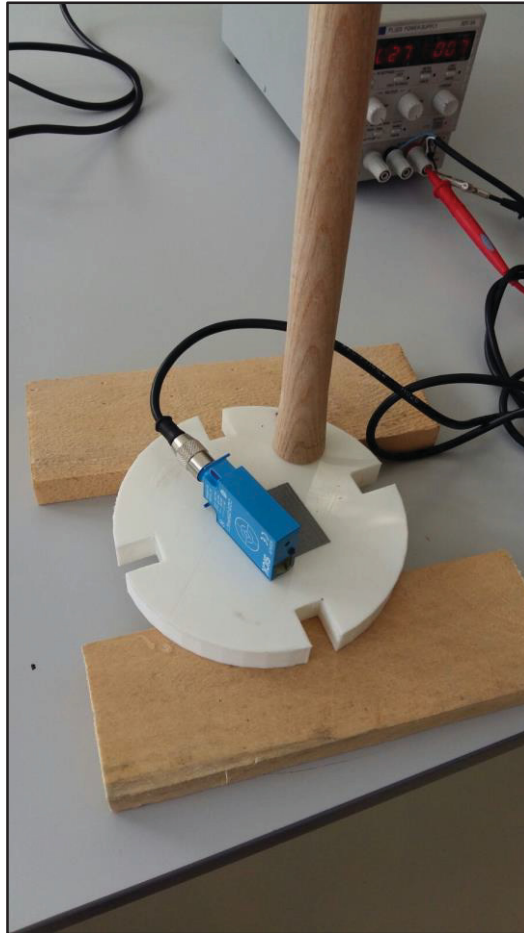
Figure 73: Insufficient sensor position for influx experiments
