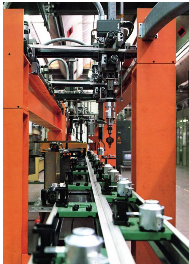
Figure 2.3: The Olivetti "SIGMA" Cartesian coordinate robot, is one of the first used in assembly applications in 1969
