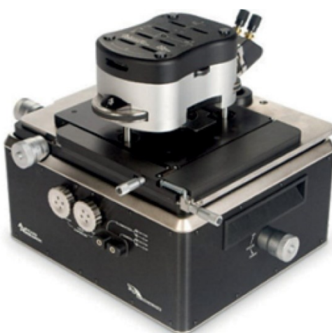
Figure 3.4: Photograph of the employed Asylum Research MFP 3D AFM.
