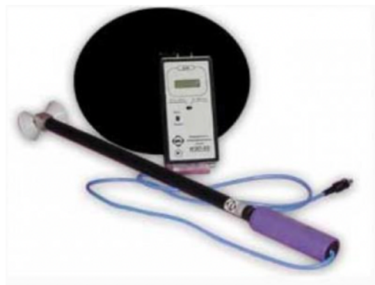
Figure 3: Electric field meter
