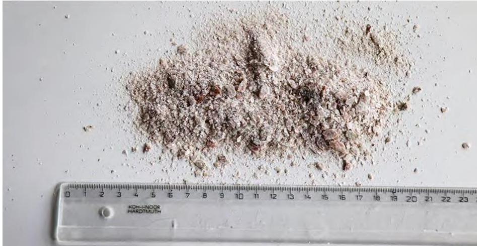
Figure 18 Cuttings from plasma-based drilling (GA Drilling a.s., 2021)
