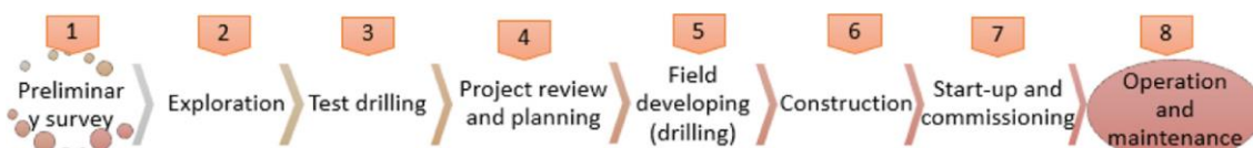
Figure 1 Schematic representation of the eight stages of geothermal development by ESMAP-WBG (D. Moya, 2018)
