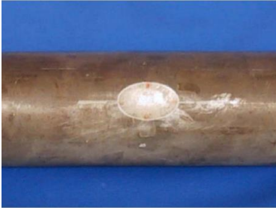
Figure 2.12 Test specimen with an induced defect
