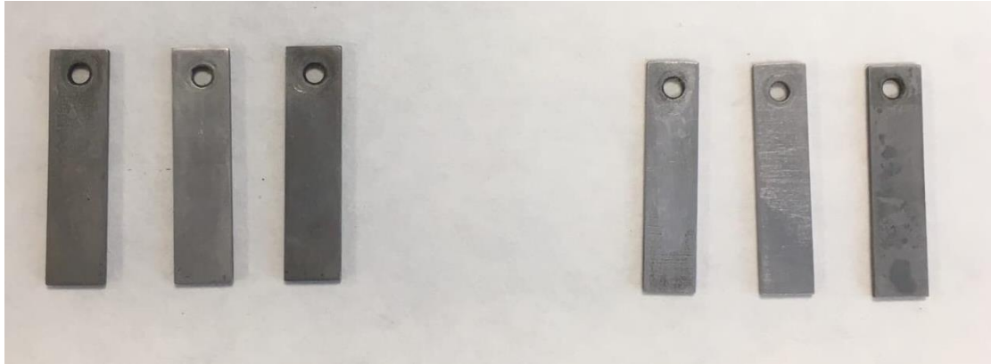
Figure 5.25: Flat metal samples made of steel St 20 after the experiment. No inhibitor (left), inhibitor injected (right)
