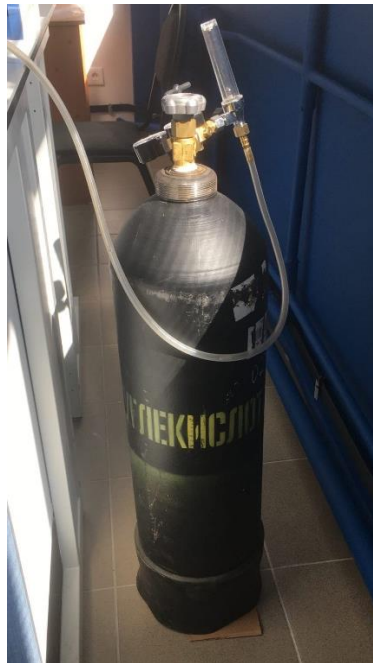
Figure 5.21: A CO 2 tank connected to the experimental unit
