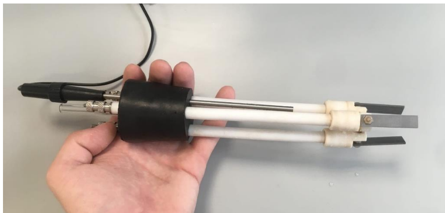
Figure 5.22: Metal samples attached to the experimental unit
