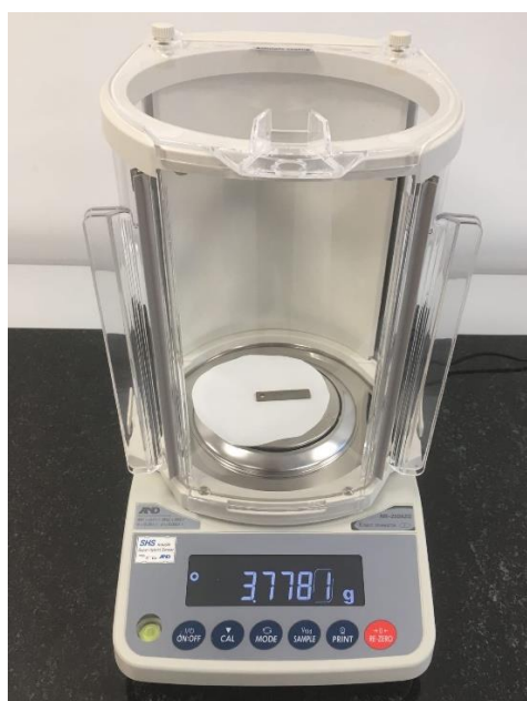
Figure 5.18: Metal sample on the high-precise analytical scales A&D HR-250AZG
