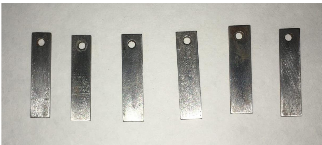
Figure 5.13: Flat metal samples made of steel St 20 before the experiment
