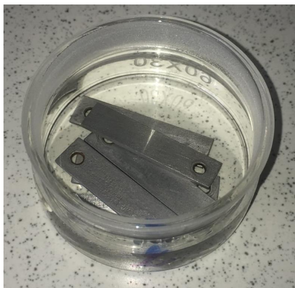
Figure 5.15: Metal samples in hydrochloric acid solution (HCl 15%)
