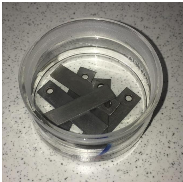
Figure 5.14: Metal samples in acetone
