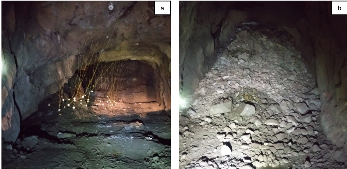
Figure 34 - Stope F410SZ041 before (a) and after (b) blasting rings 7 to 11.
