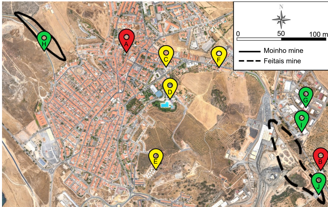
Figure 23 - Surface projection of the Feitais and Moinho orebodies and location of the monitored points within the Aljustrel mining compound.
