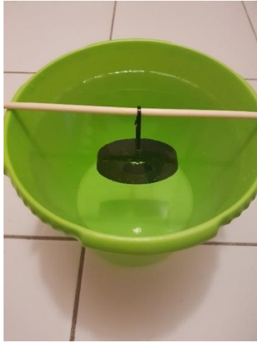
Figure 16: Magnetization by a ferrite ring-shaped magnet
