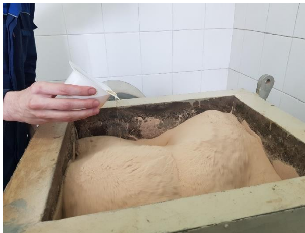
Figure 10: Adding ED-20 epoxy resin to the mixture
