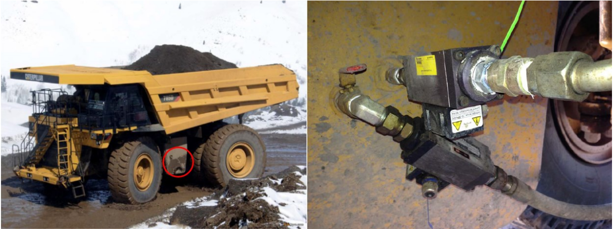
Figure 4-6 Installation of Kral Volumeters to fuel tank of Caterpillar 785D truck (Kubler & Baker, 2015).
