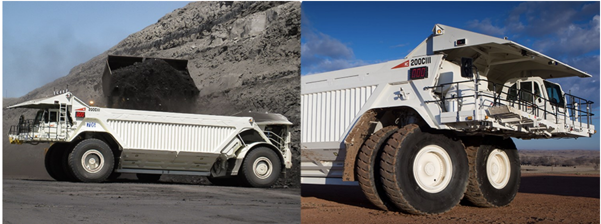
Figure 2-2 Kress 200CIII coal hauler, 220 tonnes (KRESS, 2021).
