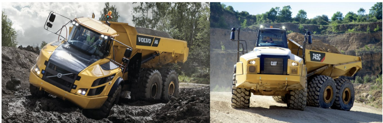
Figure 2-1 Articulated dump trucks: Volvo A40G 40 t (Volvo, 2021), and CAT 745C 41 t (Caterpillar, 2021)
