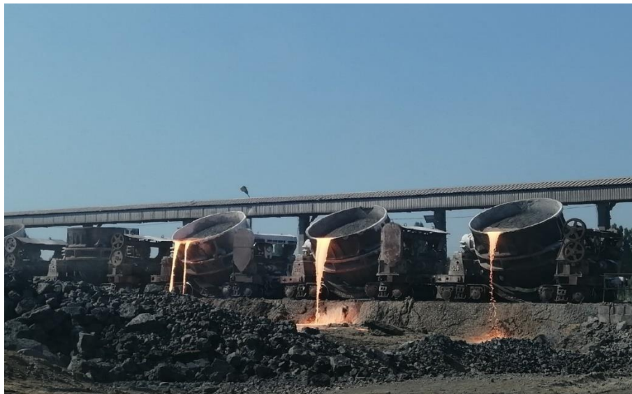
Figure 1: Drainage of liquid slag into trenches
