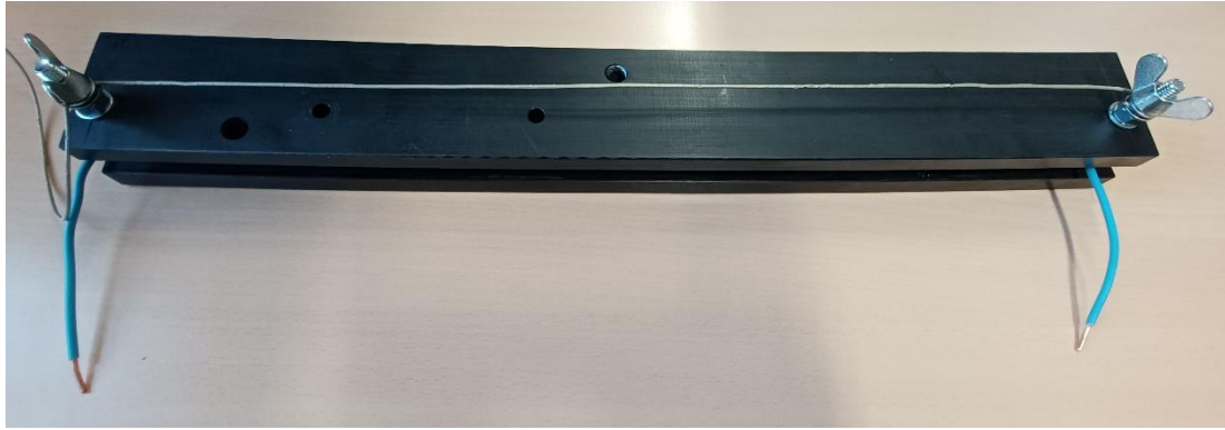
Figure 13: Measuring device for the resistances of the filaments with a specific length of 20 cm
