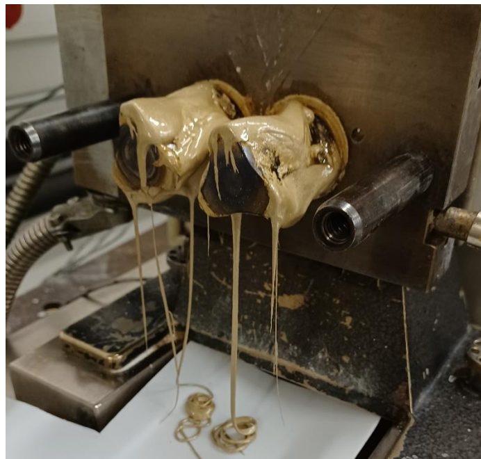
Figure 11: Open kneader chamber for mixing conductive polymer composites
