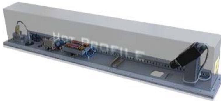
Figure 7.1: Light sectioning measurement head 1
