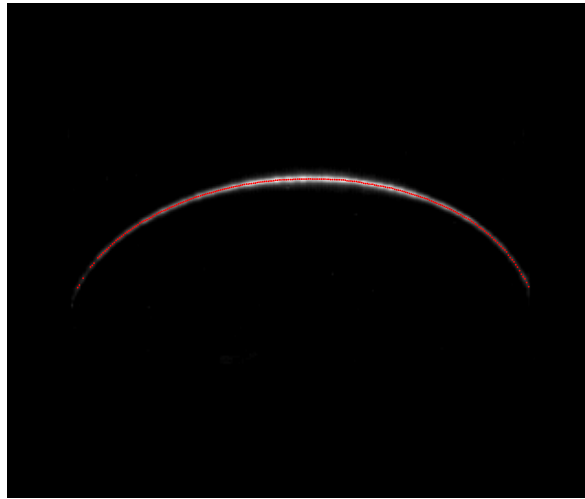
Figure 7.4: Acquired image with extracted light-section profile (red dots).
