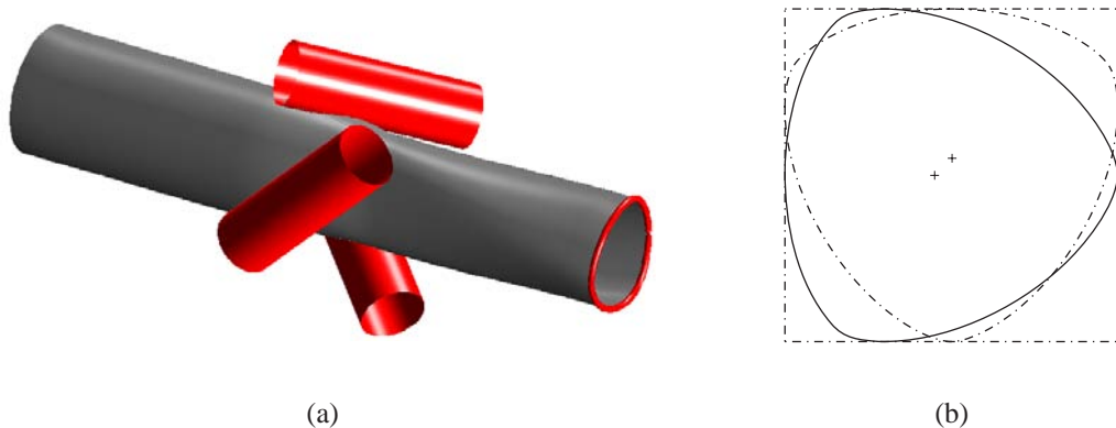
Figure 7.13: Rolling a pipe with three rolls (a); resulting profile: a curve of constant width with n = 3 vertices (b).
