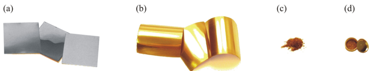
Fig. 6.2. Sample preparation steps for STA measurements to obtain film material without substrate. Low alloyed steel foils (a) coated with Ti_xZr_{1-x}N (b). Cleaned powder after chemical substrate removal (c) placed in a STA crucible with lid (d).
