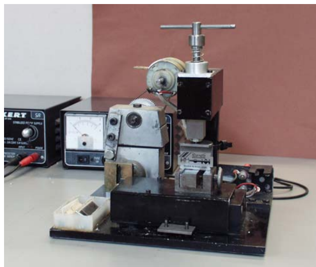
Figure 5.1: Custom-made device to produce V-notches by means of a razor blade.
