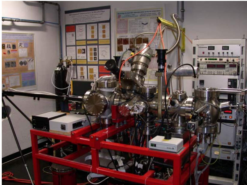
Figure 2.7: UHV system at the Institute of Physics, University of Leoben, Leoben, Austria used in this work.
