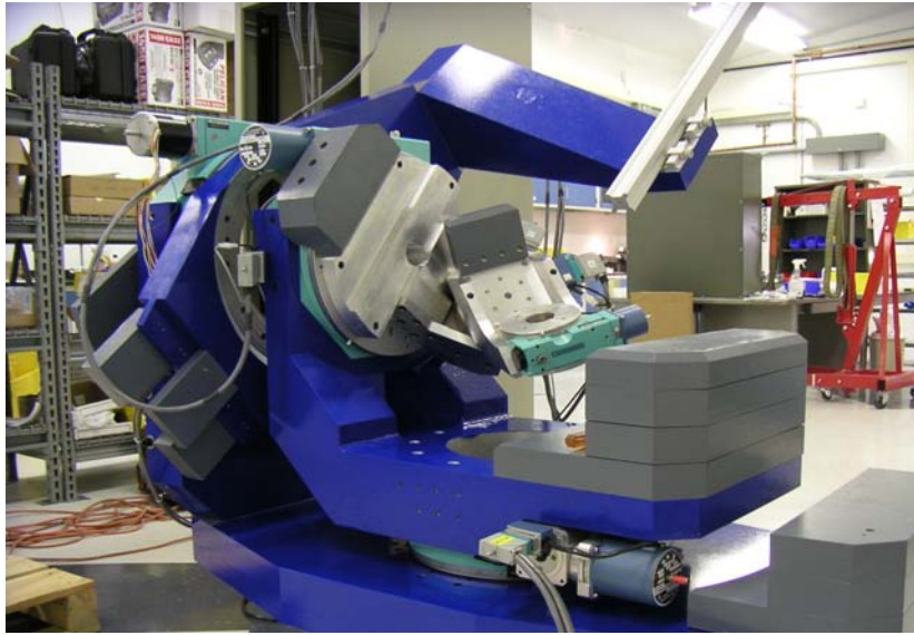
Figure 2.16: \kappa -goniometer at the G2 beamline at CHESS.
