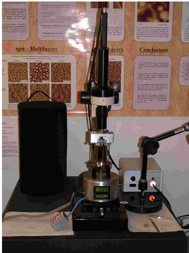
Figure 2.9: Digital Instruments NanoScope IIIa Scanning Probe Microscope used for this work, including an optical microscope for positioning the sample underneath the tip.
