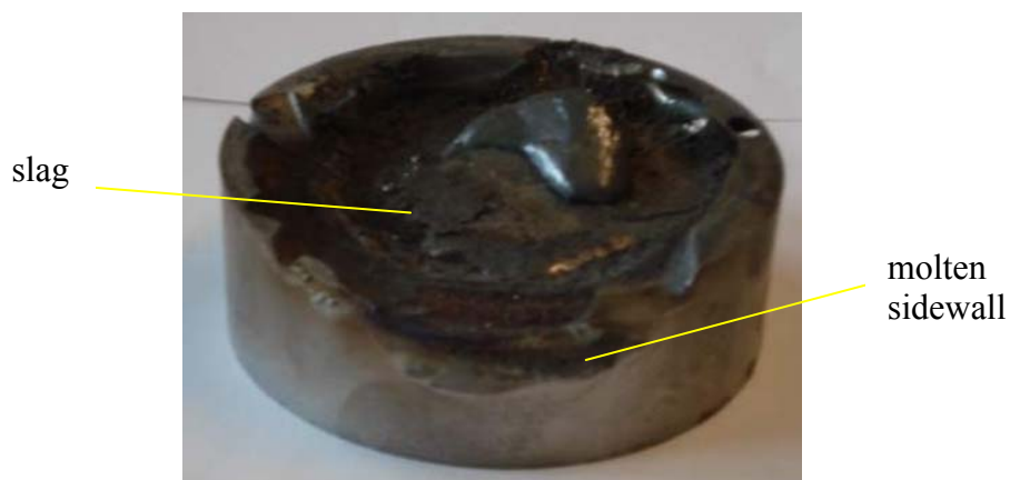
Fig. 56. Lateral shift of the arc column and melting of crucible sidewall
