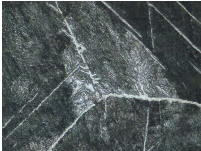
Fig. 91. Pearlite-secondary cementite structure
