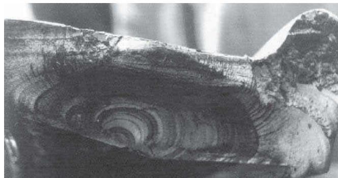
Figure 1.2: Fracture surface of the tyre of the broken railway wheel [1]
