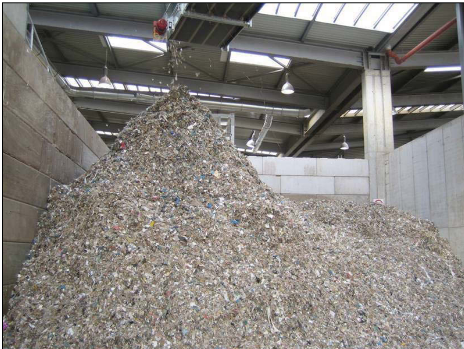
Anhang-Abb. 41: Lagerbox HOTDISC-EBS (Tageslager)
