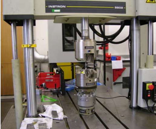
Figure 8.3: A 100 kN servohydraulic test machine and load frame.
