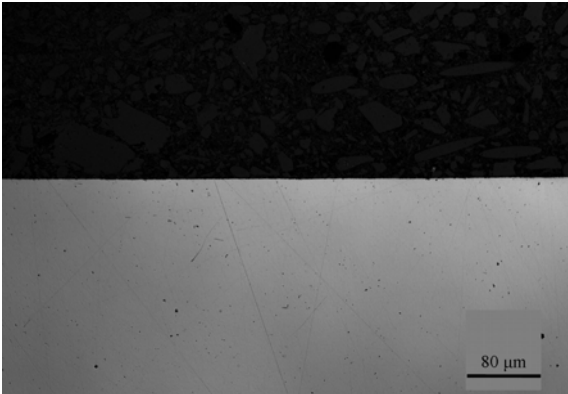
Fig. 18: Longitudinal section at the test zone of a ground specimen.
