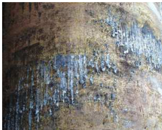
Figure 2-2: Exudations lead to the presence of high segregated Sn droplets at the surface of bronze strands in production of vertical continuous castings [RIEDLE 06].
