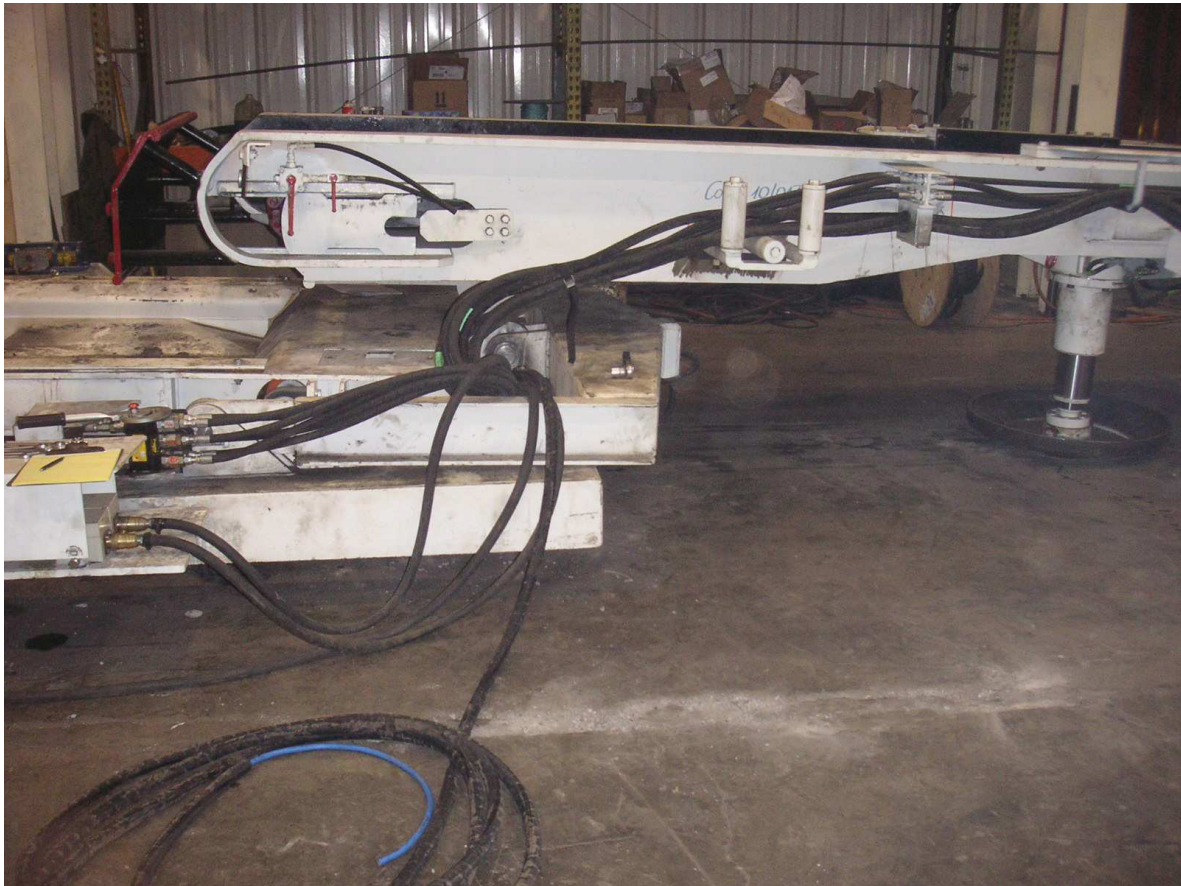
Picture 216: ABM10 – Hopper Car Hydraulic Connection
