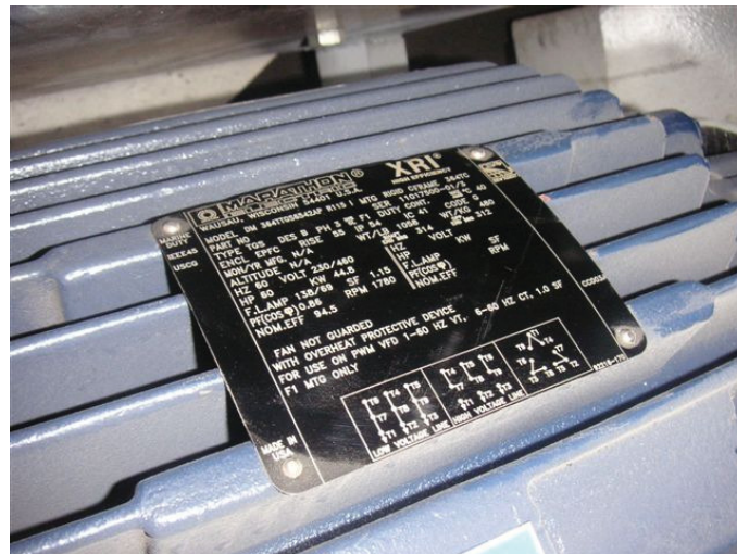
Picture 147: Specification Plate of the 45kW E-Motor
