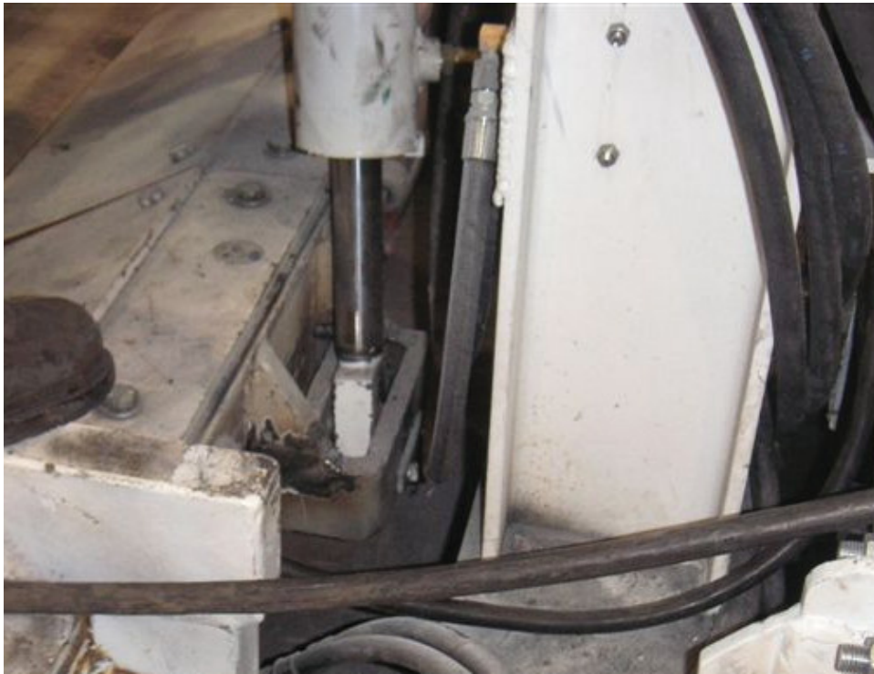
Picture 201 (cylinder new): Modified Cylinder and Clevis
