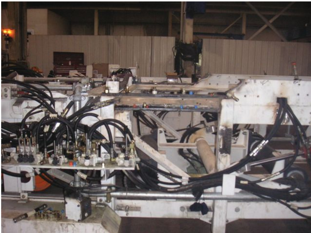
Picture 207: Carriage Frame modifications with re-arranged hydraulic components
