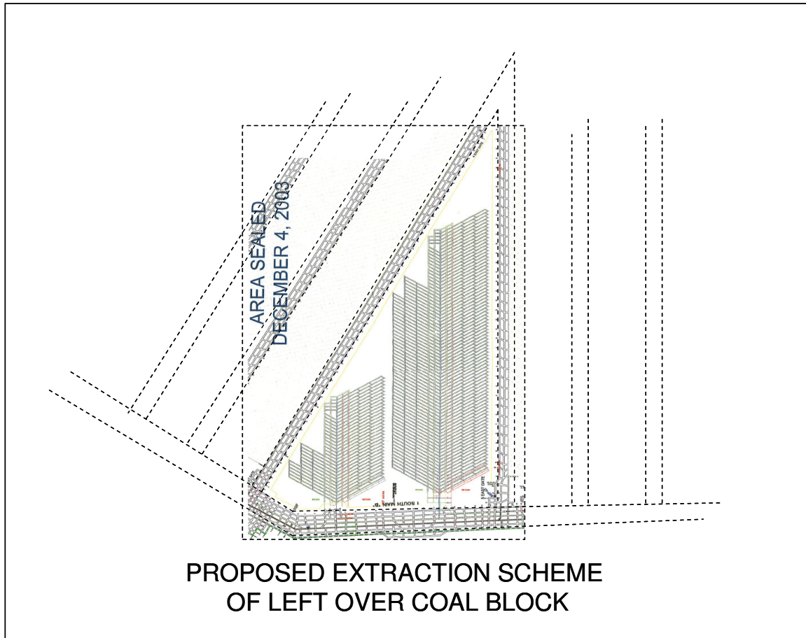
Picture 29: Proposed Room and Pillar Mining Method superimposed into the real Longwall Mining Operation
