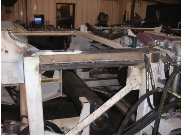
Picture 205: Carriage Frame modifications
