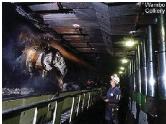
Picture 11: Longwall Shearer / Hydraulic Supports; Source History and Methods of Longwall Mining, www.uow.edu.au/eng/longwall/history.html
