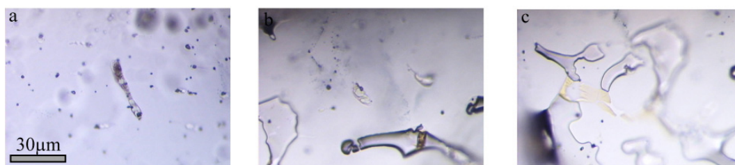
Fig. 5.3. Inclusions and unhealed cracks containing various solid phases, formed in experiment 005.
