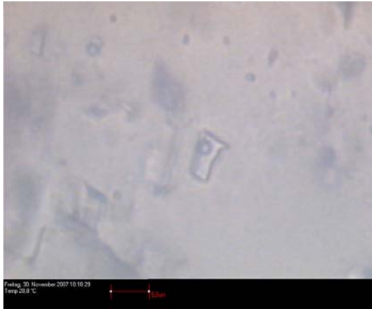
Fig. 6. 3 Primary two-phase aqueous inclusion with a vapour bubble and a liquid (sample No. M2-PI).
