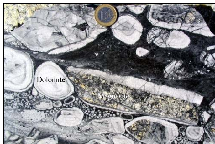
Fig. 3. 27 Orbicular dolomite composed of light dolomite spheres and pinolite magnesite as cores.
