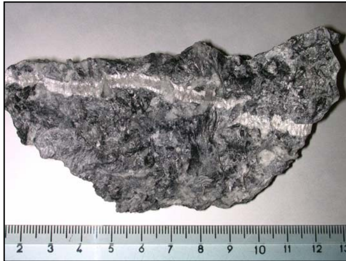
Fig. 3. 31 Fibrous aggregates of talc along a joint.
