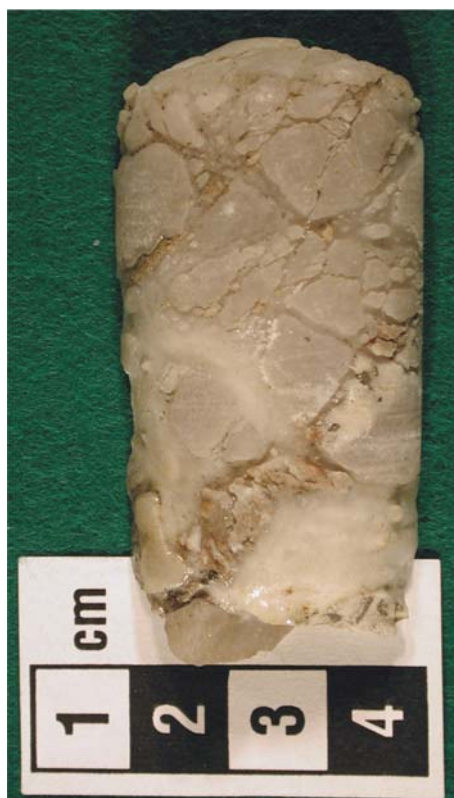
Fig. 5. 7 Gypsum and anhydrite drill core which was intercalated within magnesite host sediments in NW underground parts of the deposit.
