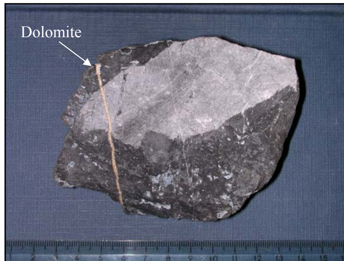
Fig. 3. 30 Dolomite as joint fillings is interpreted as the youngest dolomite generation.
