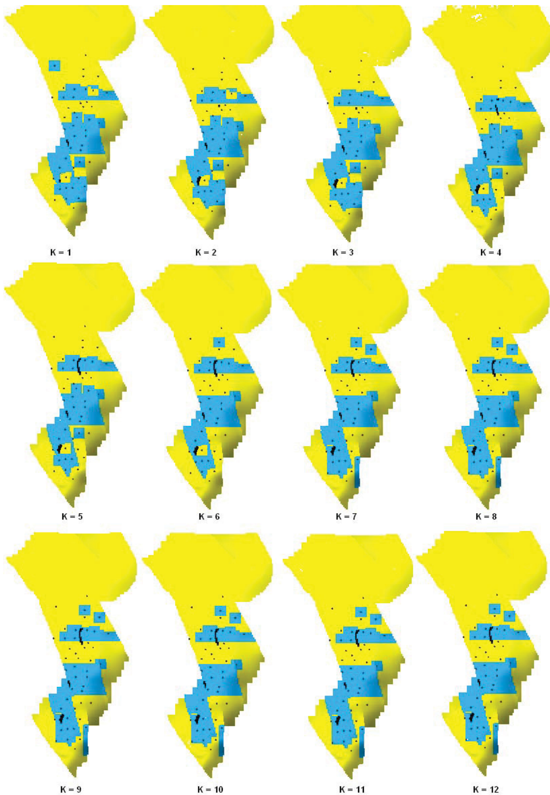
Figure 6.4: Lateral permeability alterations in HM model (yellow - no change, blue - changed, dots - wells).
