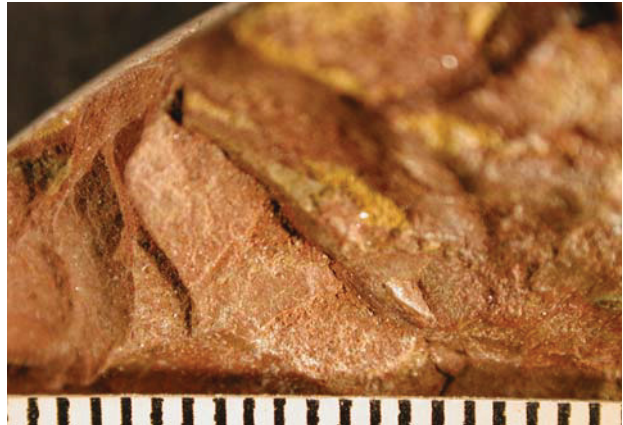
Fig. 8.11a: AW14 of Core II of the Amir Wali Well at 1615.06 m, firm and indurated claystone.
