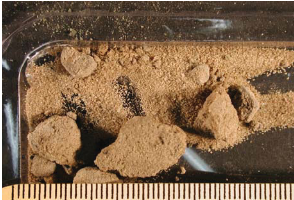
Fig. 8.2a: AS 29 of Core III of the Ali Sahib Well at 1731.0 m, loose sand to friable sandstone.
