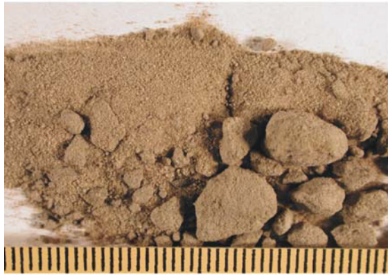
Fig. 8.3a: AS 30 of Core III of the Ali Sahib Well at 1731.60 m, loose sand to friable sandstone.
