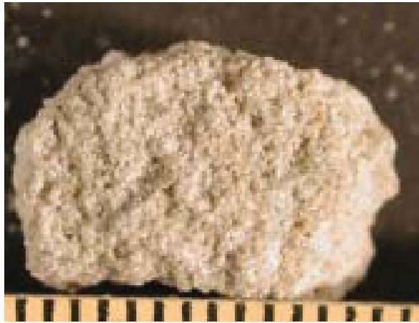
Fig. 8.16a: AW20 of Core II of the Amir Wali Well, at 1621.20 m, friable sandstone.
