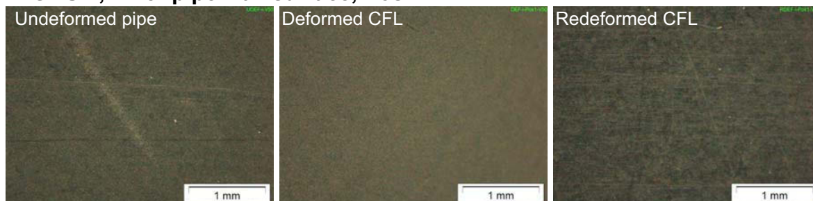
Fig. 10.1: Outer and inner pipe wall surface of the undeformed pipe, the deformed CFL and the reformed CFL at Pos. 1 of AGRU II.
