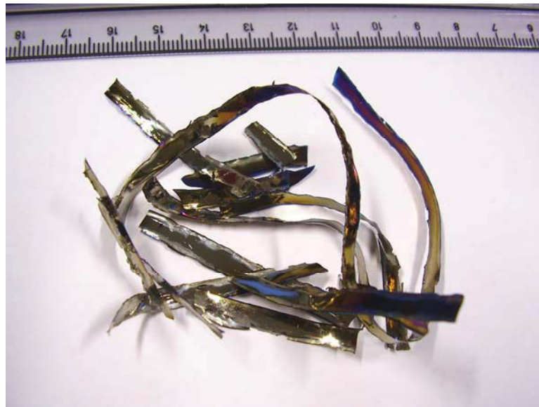
Fig. 3-7: The brittle melt-spun ribbons occurred after reaction between NiTi alloy and quartz crucible at temperatures above 1400 °C.
