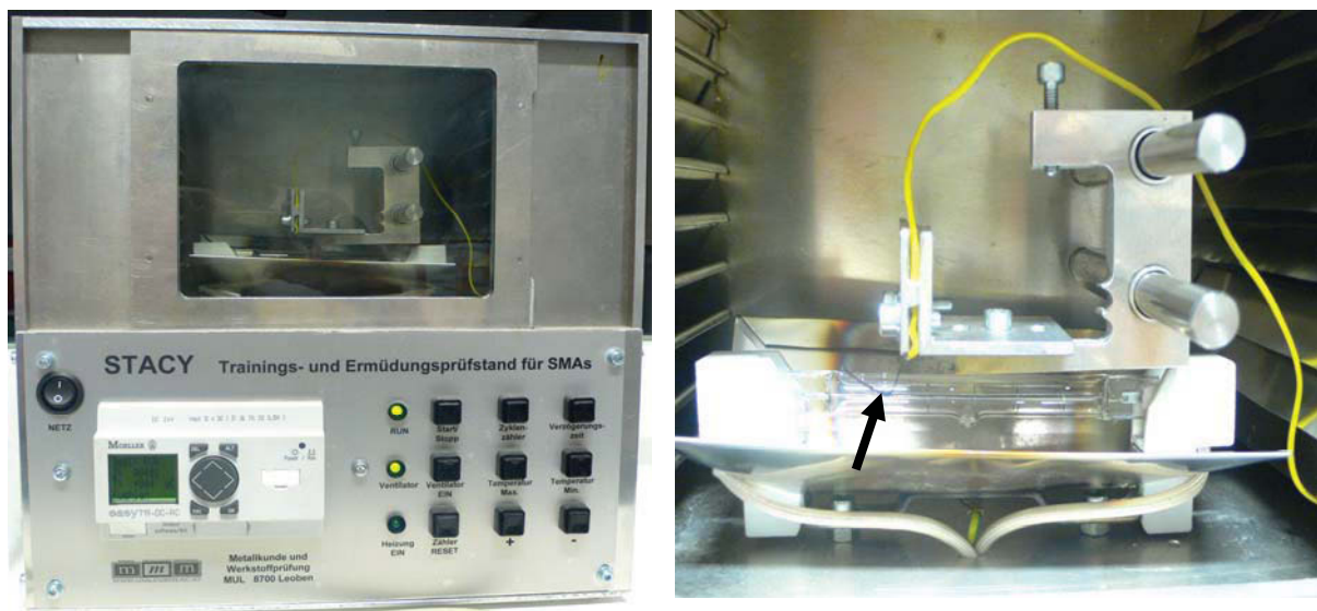
Fig. 3-15: (a) Self-fabricated bending training device (b) close-up of samples holder showing the trained ribbon (arrow).
