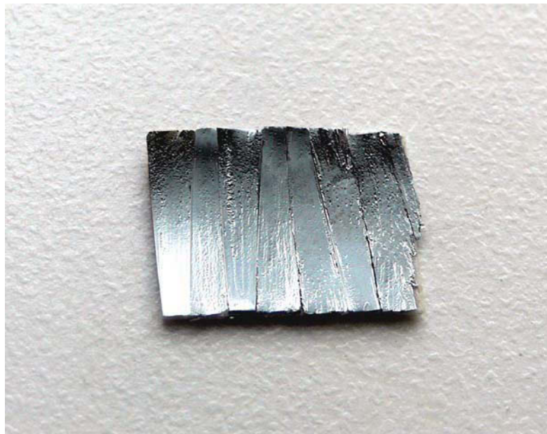
Fig. 3-12: A melt-spun ribbon fixed on the glass sheet for the XRD investigations.
