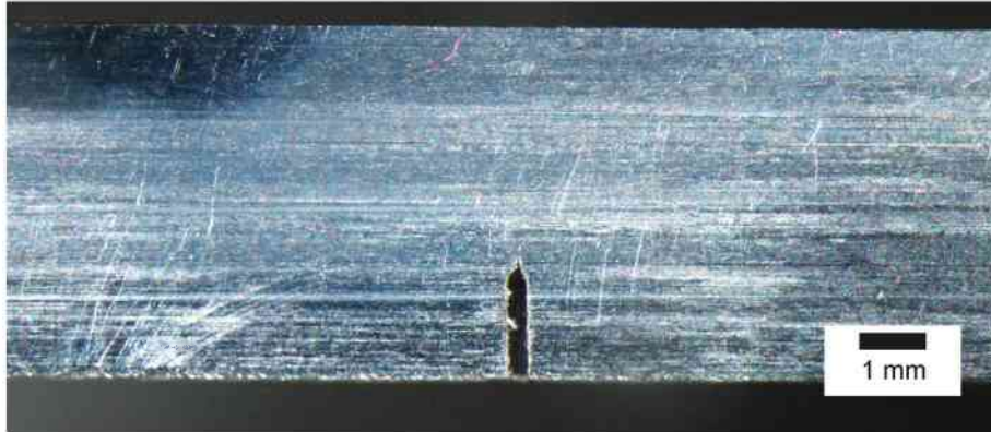
Fig. 5.6 Photograph of Al7075/Al1050 fracture mechanics Specimen 2 before testing.
