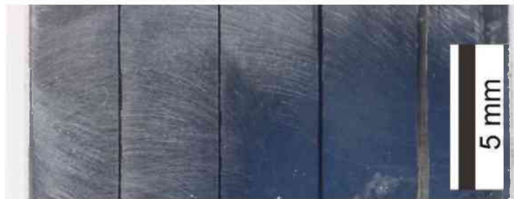
Fig. 4.11 Photograph of the Al7075/Adhesive multilayer.
