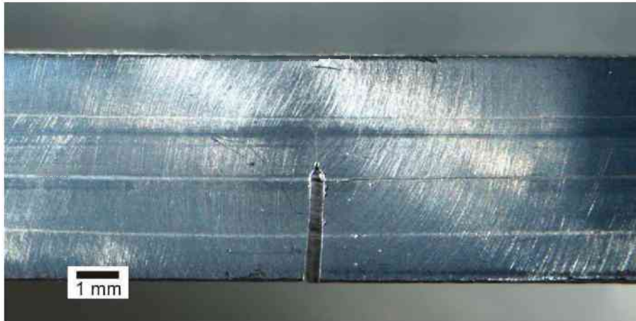
Fig. 5.2 Photograph of Al7075/Al1050 fracture mechanics Specimen 1 in the unloaded state.
