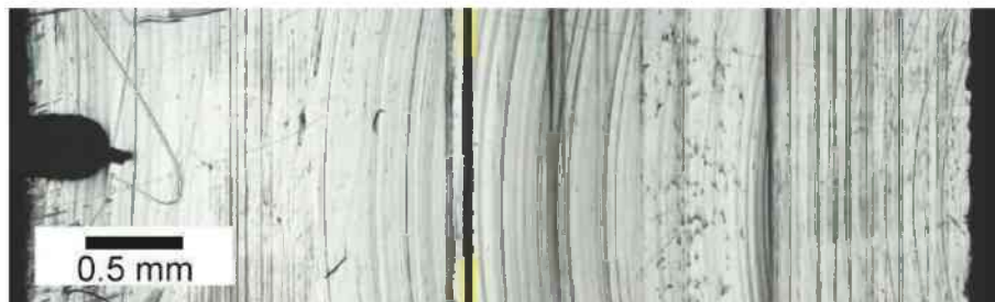
Fig. 6.8 The notch tip area of Al7075/Adhesive Specimen 2 with the interlayer at 0.5W . The interlayer location is marked by yellow lines.
