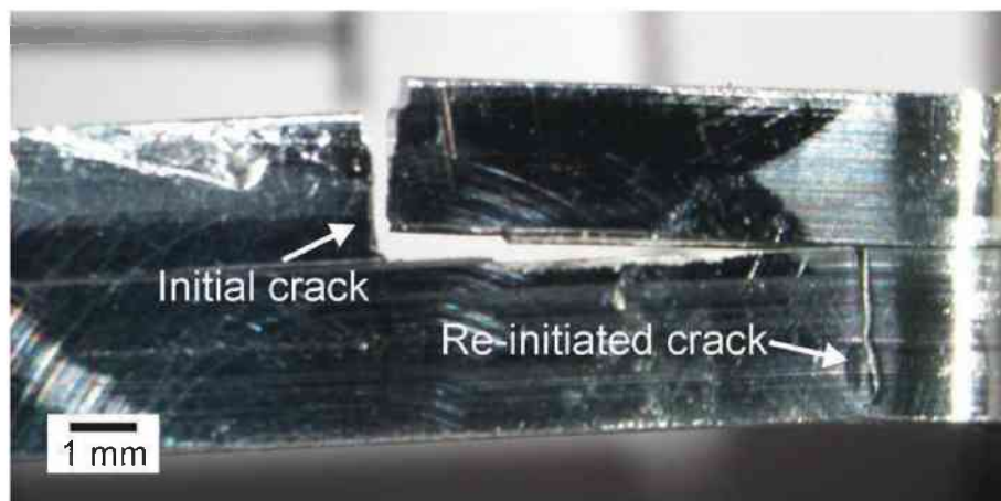
Fig. 6.11 Al7075/Adhesive Specimen 2 after re-initiation of fatigue crack growth in the second stiff layer.
