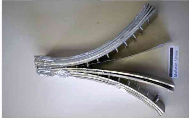
Fig. 4.15 Alligatored Al7075/Al1050 stack for roll bonding. The fractured aluminum rivets are clearly visible.
