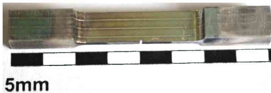
Fig. 4.19 Notched and etched Al7075/Al1050 fatigue specimen with 4 hard and 3 soft layers.
