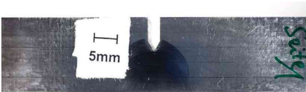
Fig. 6.3 Photograph of Al7075/Adhesive Specimen 1 before testing. A magnification of the notch tip is shown in Fig. 6.4a.
