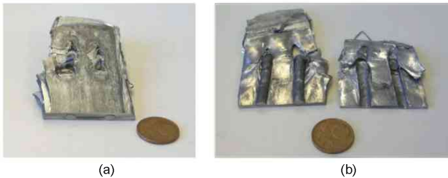
Fig. 4.16 Al7075/Al1050 stack connected with iron rivets after roll bonding. Cracks formed at the interface rivet/aluminum inhibiting bonding.
