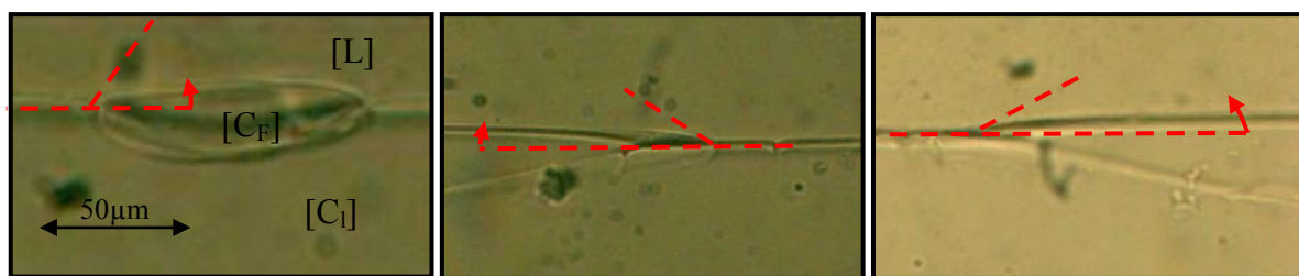
Figure 67 : Wetting angle \Phi between the secondary and the primary phase. The solid/liquid interface is indicated by the red broken lines.
