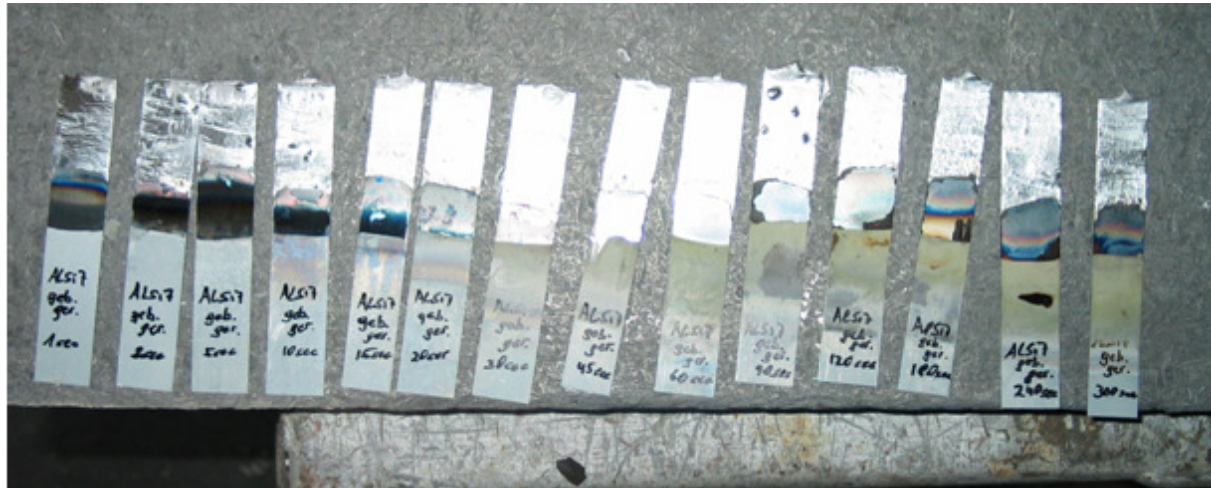
Figure 14: Steel strips dipped into a binary Al-Si7 alloy with dipping times ranging from 1 s (left) to 300 s (5 min, right)
