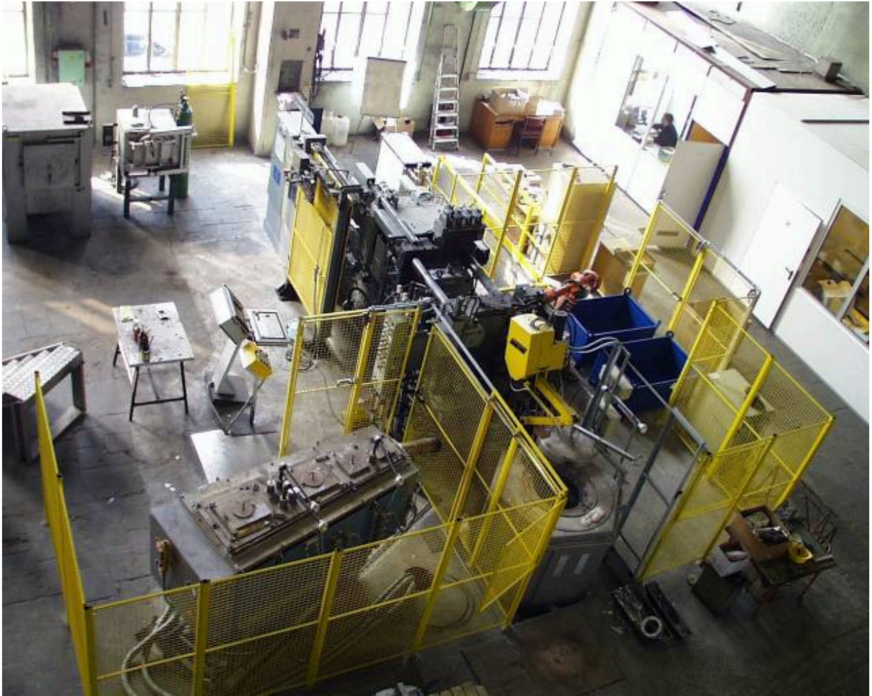
Figure 15: UBE HVSC 350 t squeeze casting (SCQ) machine with dosing robot
