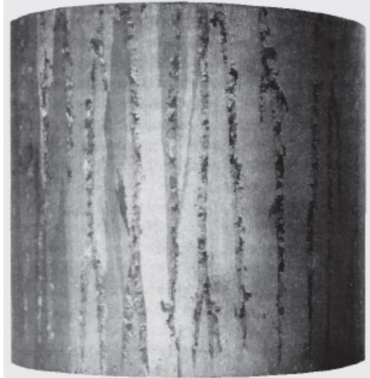
Figure 2.3: Freckles at the surface of a 0.1 m diameter cylinder of a MAR-M200 superalloy [42].
