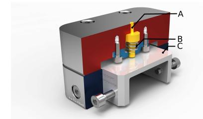
Figure 2.1: Rendered section view of the acoustic actuator which is installed in the test mold. The actuator consists of a sprung movable pin (A) which is pushed by a spring (B) in the cavity. The movable pin is accelerated by the melt front towards the resonant body (C) on which it impinges generating a structureborne sound with a unique frequency pattern depending on the resonator's shape.
