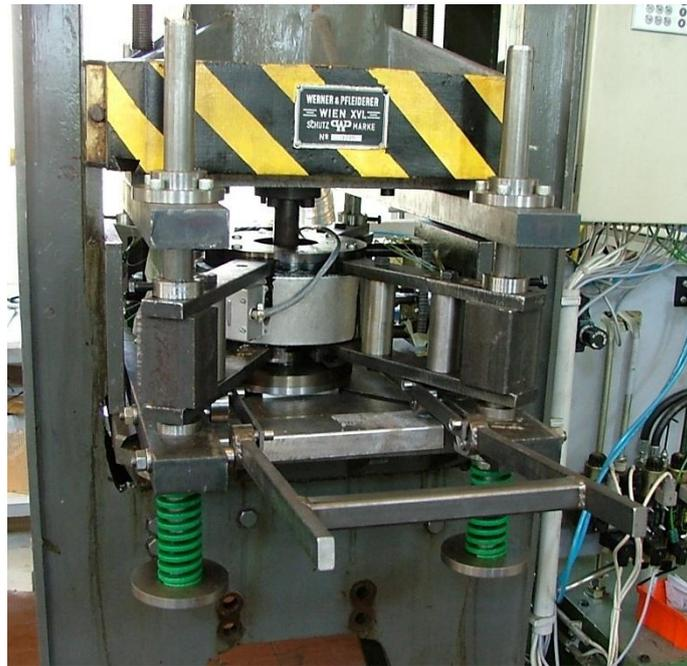
**Figure 3.4:** Experimental extruding plant during application: Remarkable is the heating sleeve (light grey colour, in the centre) around the mantle. The maximum press speed of the adapted hydraulic 100 ton press is 7 mm/s.
