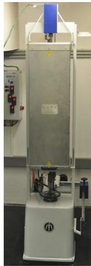
**Figure 3.7:** Creep furnace used for short term creep tests at constant load.
