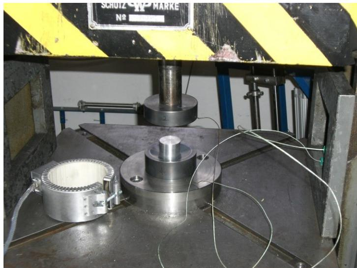
**Figure 3.6:** Experimental set-up to perform the spike test series. In the centre, upper and lower die with the aluminium billet and thermocouples are apparent. The heating sleeve in the left was used to heat up the tools to working temperature, the aluminium billet was preheated in a furnace.
