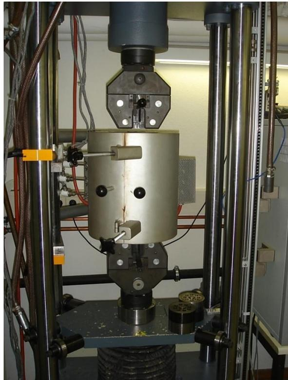
**Figure 3.8:** Testing device for cyclic loading conditions, which was used to perform the experimental fatigue as well as the creep-fatigue test series.
