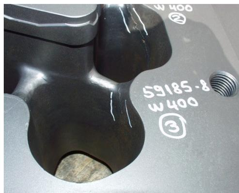
**Figure 1.1:** Damage observed in a W400 extrusion die. The cracks are marked with white lines.
