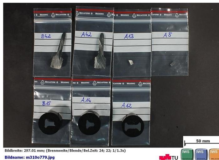
**Figure 5.57:** Creep as well as fatigue and creep-fatigue specimens prepared for dislocation density measurements with X-ray diffraction peak profile analysis.
