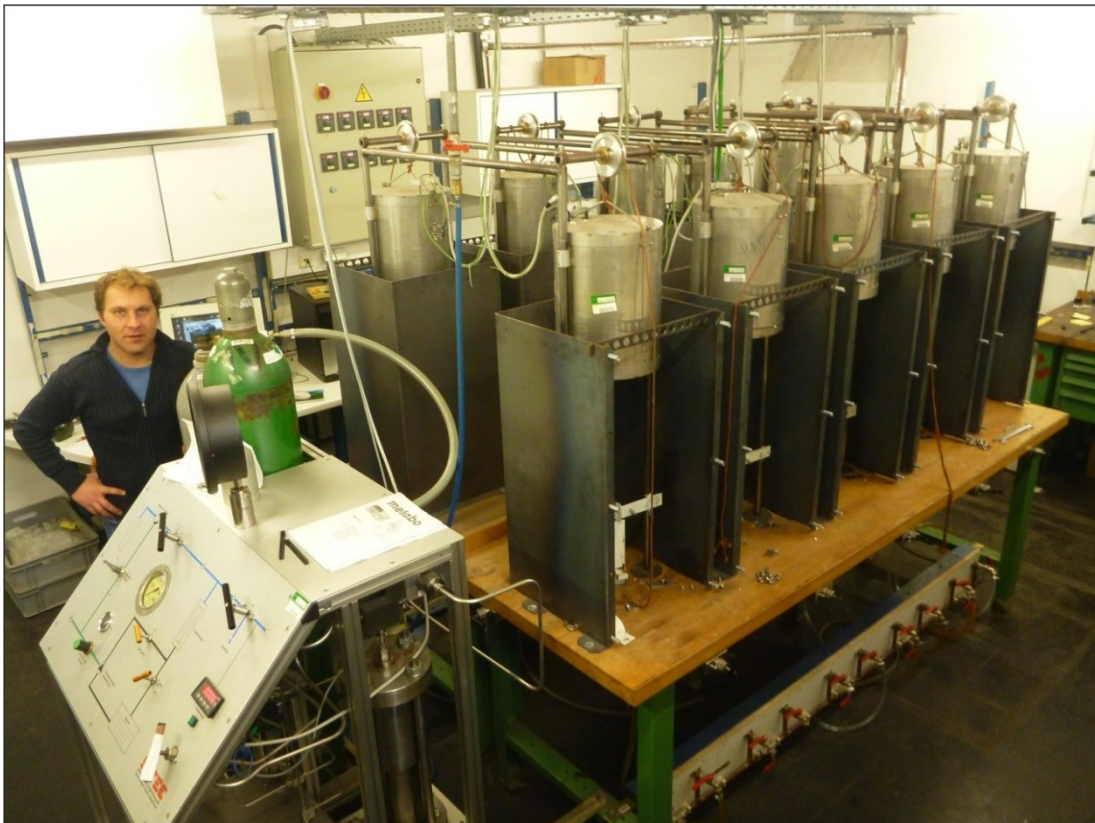
Fig. 1 High pressure / high temperature hydrothermal laboratory device in Leoben
