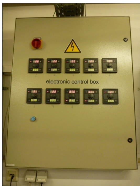
Fig. 12 Electronic control box which is interposed between the furnace and the computer software for digitalizing the electronic signal of the furnace
