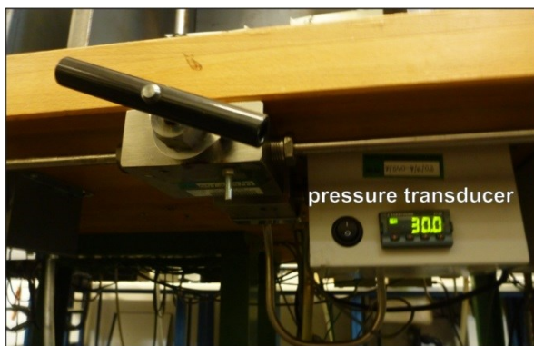
Fig. 5 (top left) UHP tube-system with a valve and the interposed pressure transducer
