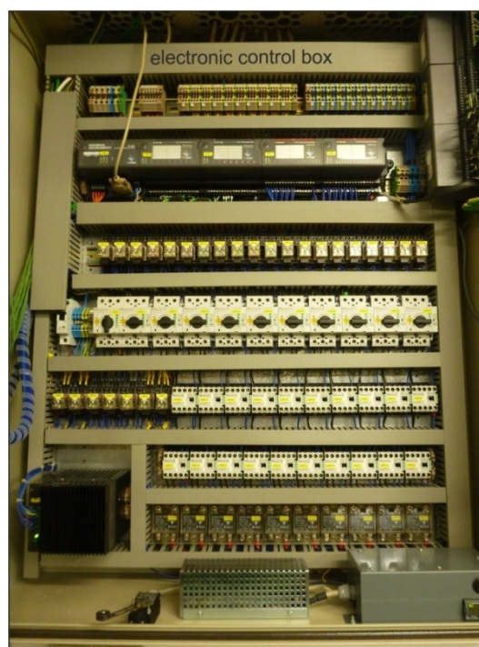
Fig. 12 Electronic control box which is interposed between the furnace and the computer software for digitalizing the electronic signal of the furnace
