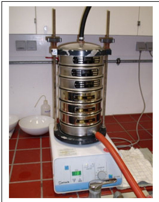
Figure 17: Wet sieving process applied
