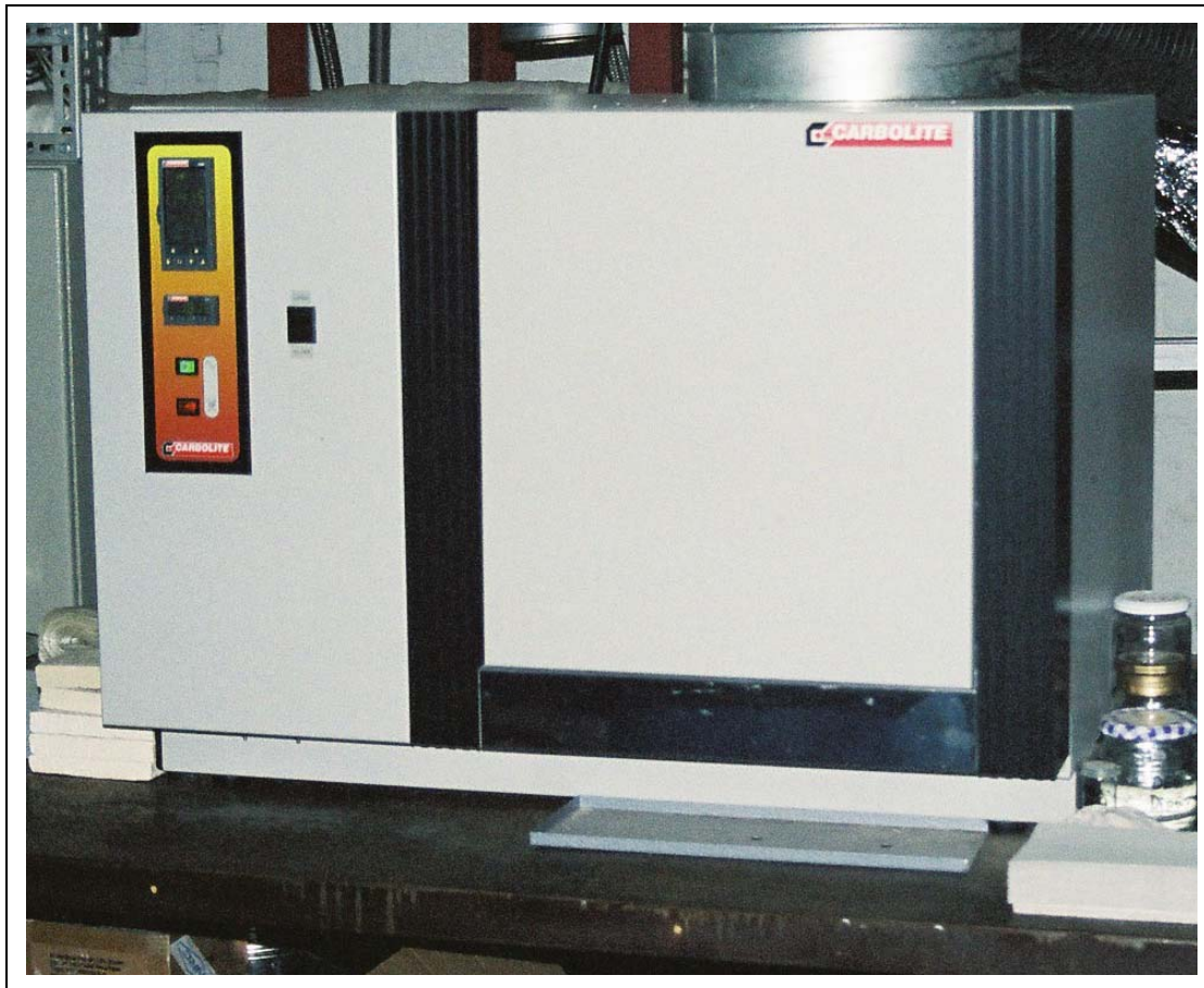
Figure V-1: Carbolite sintering oven (general view)
