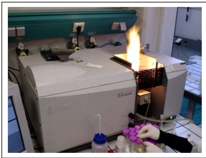
Figure 15: Flame AAS equipment used
