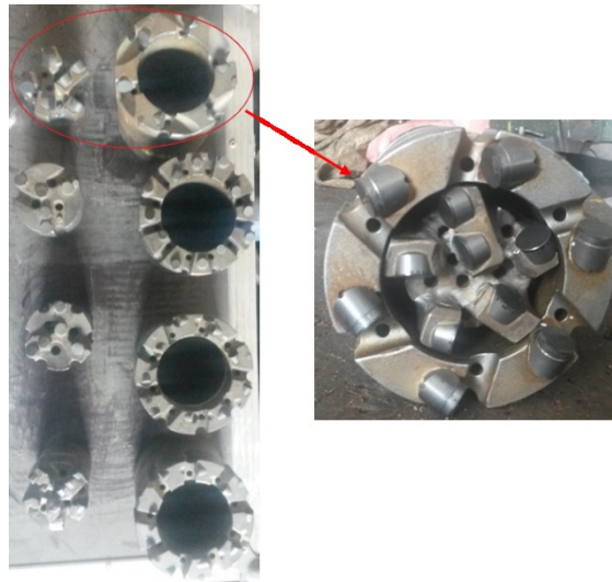
Figure 6-11 2nd pilot and reamer: larger cutter size which leads to lower MSE
