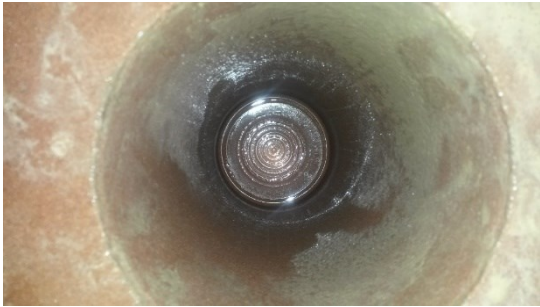
Figure 6-9 Smooth bottom hole, indicates very low vibration frequency/rate
