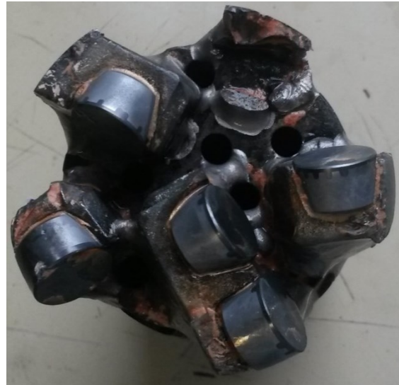
Figure 6-23 Broken cutter (test 9)
