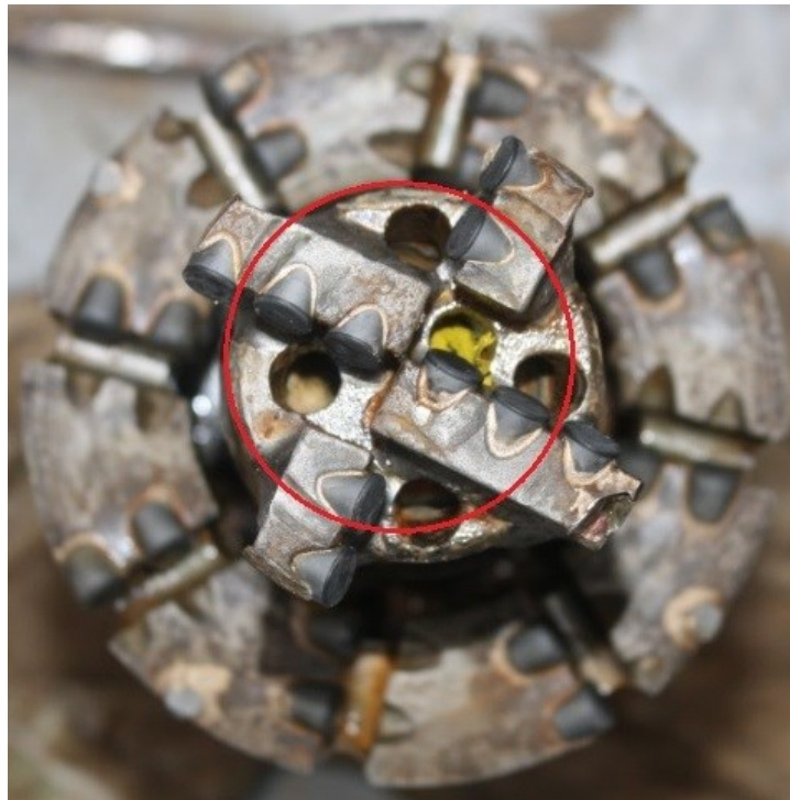
Figure 6-8 Wear ring on body bit indication of high WOB
