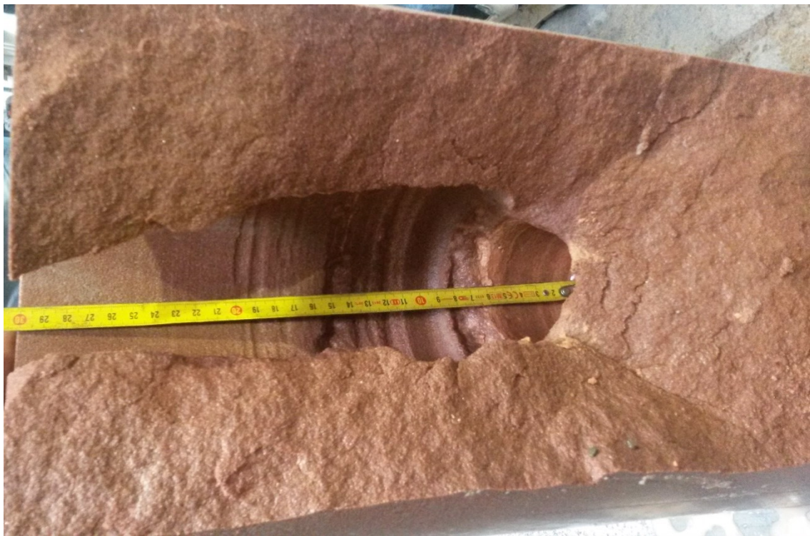
Figure 6-24 Extreme vibration while rotating off bottom (test 8), unsmooth wellbore is a good indication of vibration
