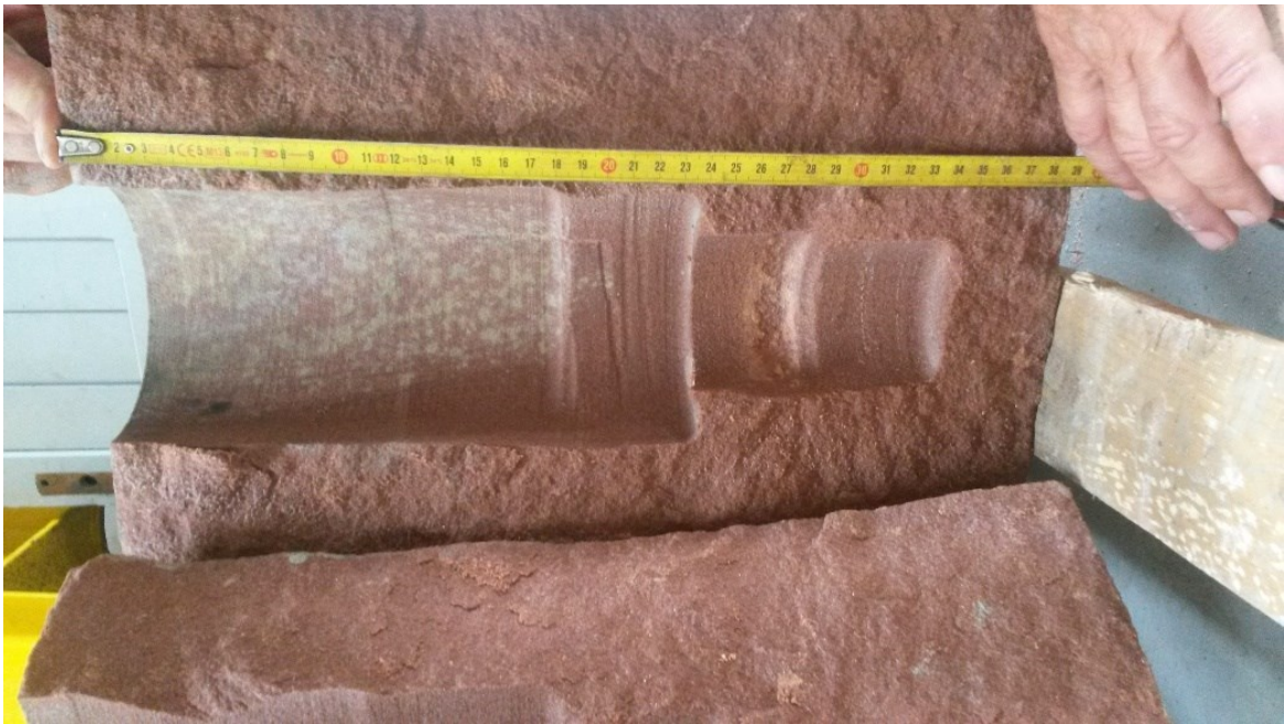
Figure 6-17 The sample was enlarged and broken due to long period of time off-bottom rotation at the same depth
