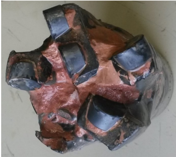
Figure 6-22 the pilot bit balling (test 9)
