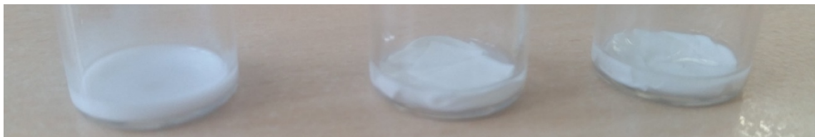
Figure 2.4. Solubility of PET 1 after ageing at 125°C, left: 1000 h, middle: 2000 h, right: 3000 h.
