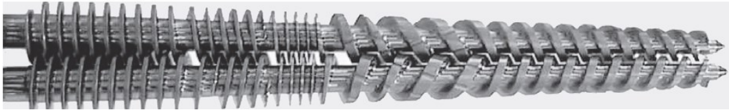
Figure 19: Conical, intermeshing screws variation [23].
