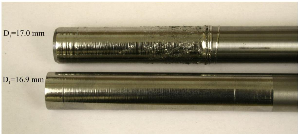
Fig. 65: Sample  $D_1 = 17.0$  mm &  $D_1 = 16.9$  mm after ball spinning.
