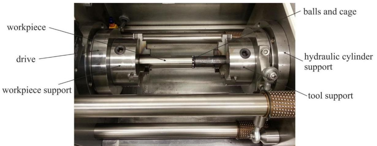
Fig. 39: Experimental setup of the friction welding machine.
