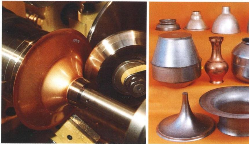
Fig. 3: Spinning and shear spinning products (Runge, 1993).
