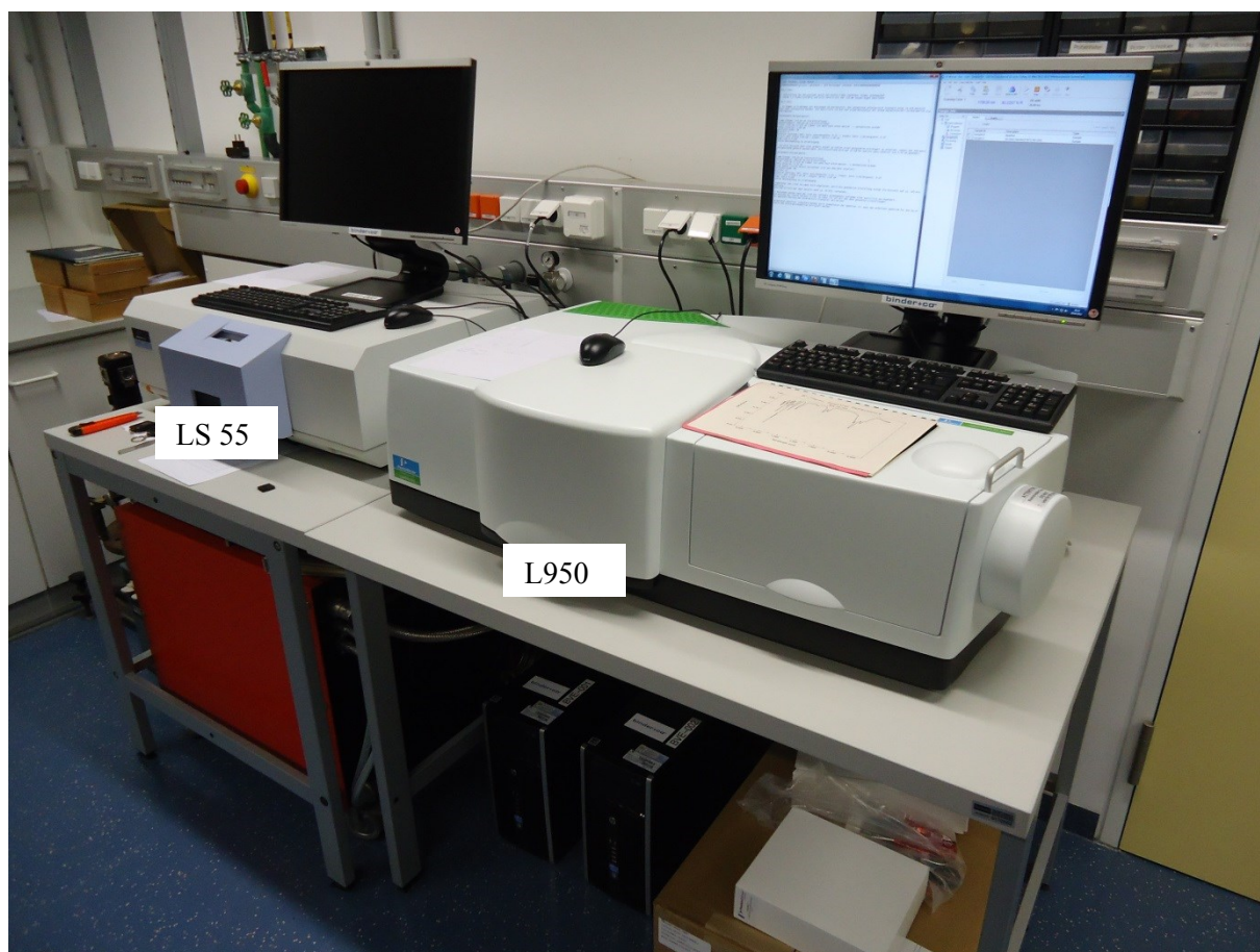
Fig. 61: Setup for optical measurements: LS 55 Luminescence spectrometer and L950 reflection spectrometer (TU-Graz)
