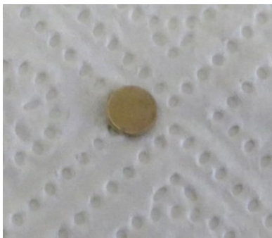
Fig. 28: Metallized oxalate product pellet for IS-analysis
