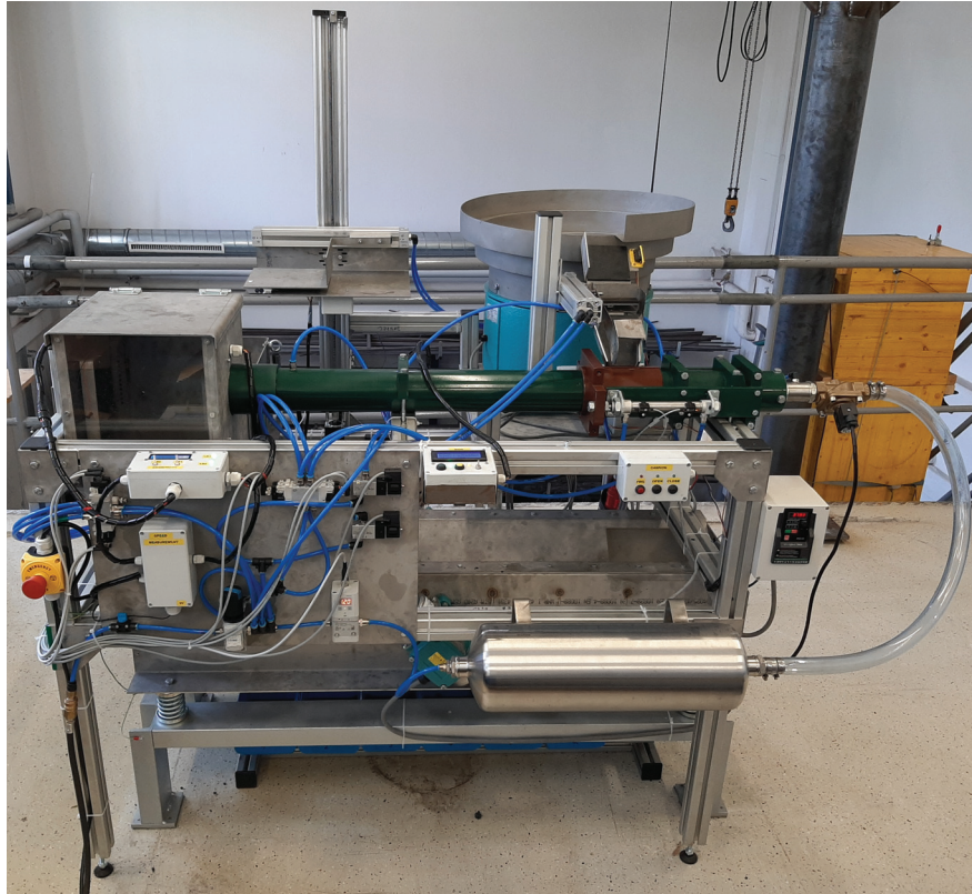
Figure 6.7: Automated test rig for rapid single particle impact testing to determine sinter breakage behavior [1]
