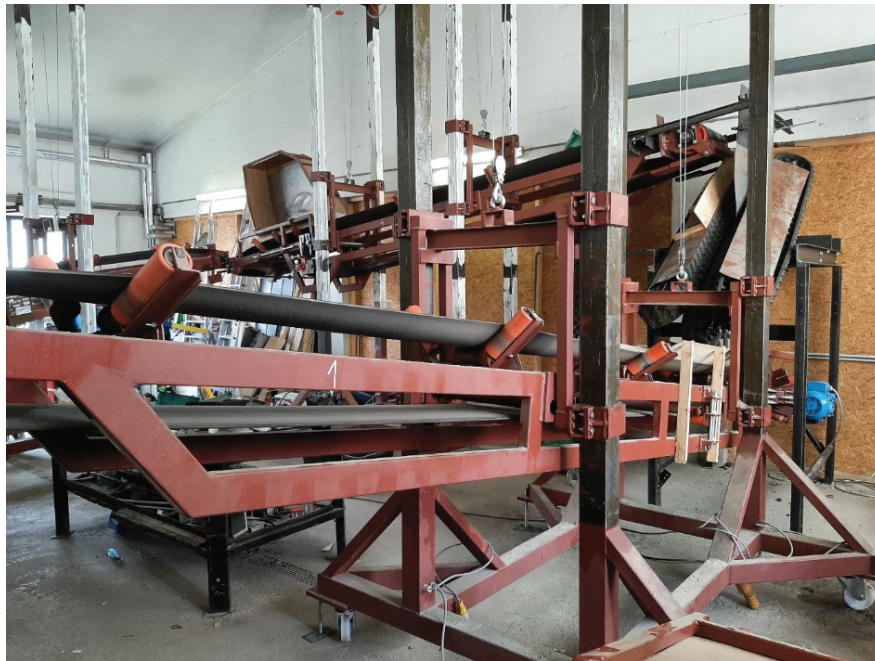
Figure 7.4: Conveying circuit with operating FlowScrape [5, 11]
