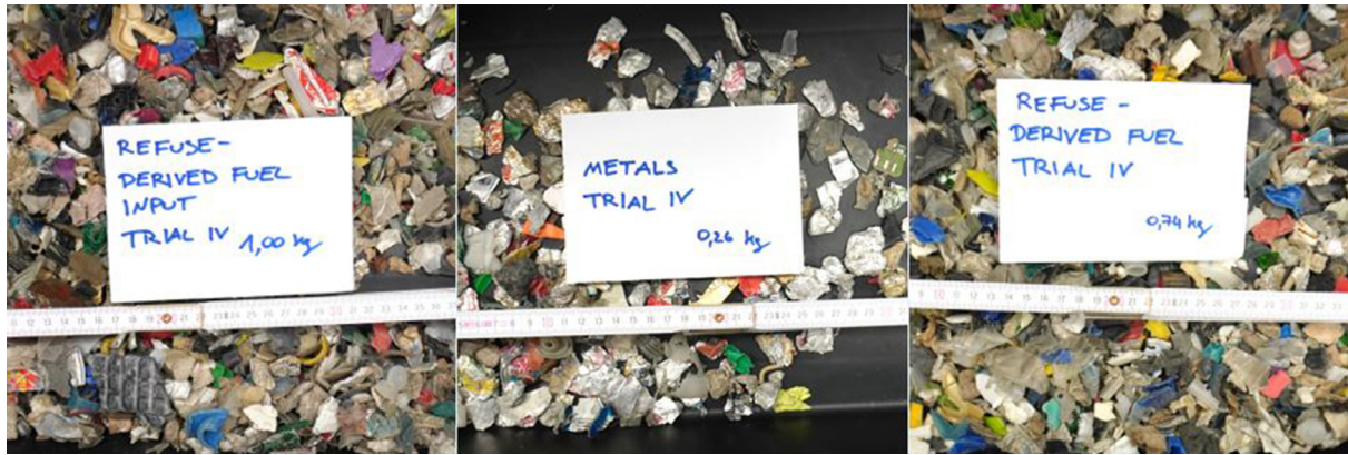
Fig. 15. Feed material (left), separated metal – Eject (centre) and refuse-derived fuel – Reject (right) (Trial 4 of Table 9) (authors depiction).
