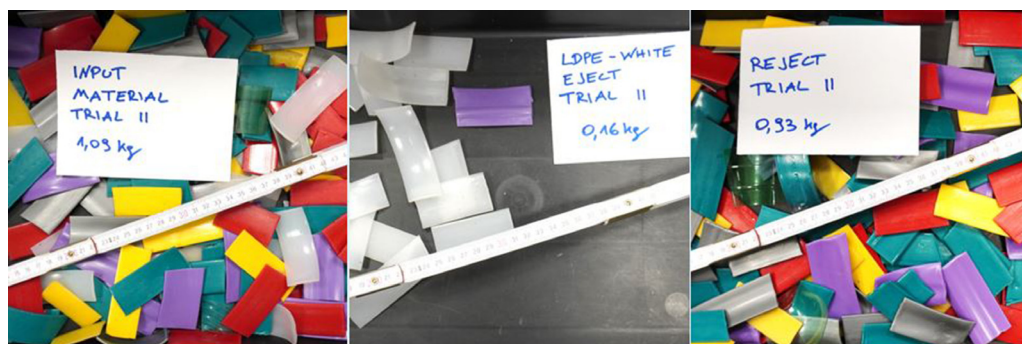
Fig. 5. Feed material (left), separated white LDPE – Eject (centre) and coloured plastic – Reject (right) (Trial 2 in Table 5) (authors depiction).
