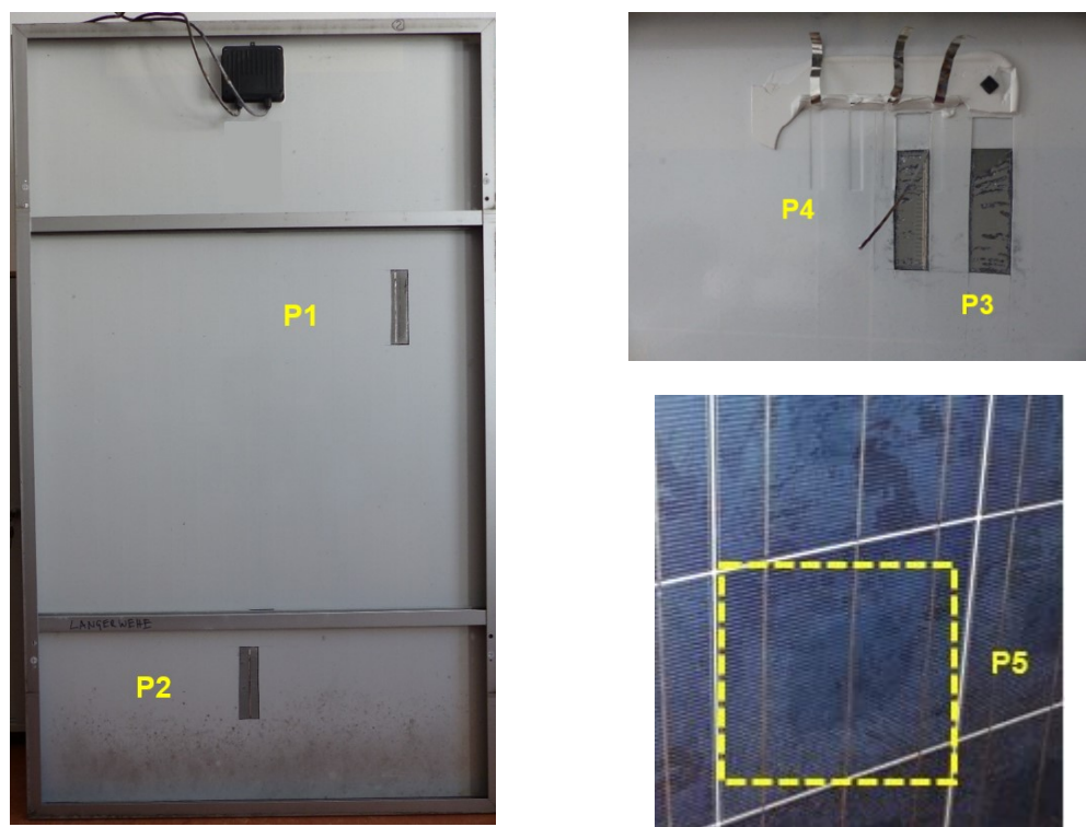
Figure 6.1: Positions of encapsulants' withdrawal. P1 and P2 (left): back encapsulant, in contact with the cell and the backsheet, indirectly exposed to outdoor conditions. P3 (top right): back encapsulant between cell and backsheet, below the adhesive layer connecting the junction box. P4 (top right): back encapsulant between cell and
