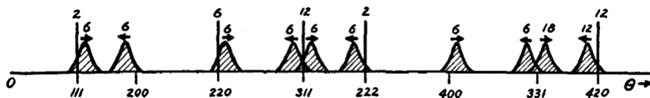
Figure 36: Indication of the direction of the peak shifts caused by planar faults [112].
