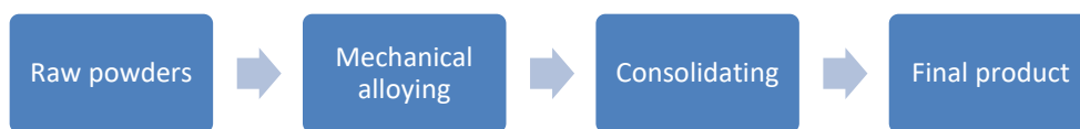
Figure 9: Schematic illustration of the process route for the production of ODS-materials via mechanical alloying.
