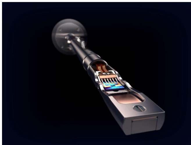
Figure 2.11: Protochips Fusion Select holder for TEM, clearly showing the comb of electrical contacts touching the e-chip [88]
