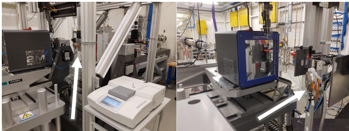
Figure 3.7: Experimental setup for the in-situ synchrotron measurements, showing the measurement cell where the chip is mounted outside of the FDSC device and in the path of the beamline.
