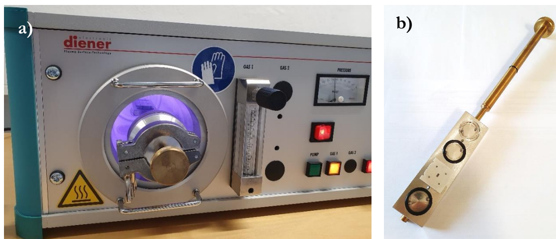
Figure 3.4: a) Plasma cleaner from Diener electronic GmbH with a custom holder for MultiStar FDSC 1 chip sensors. The holder (b), where chips are placed onto rubber O-rings and two small anchoring posts.
